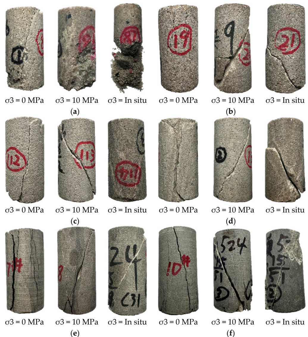
Figure 3. Post-test failure morphologies of the three sandstone types under different confining pressures: (a) CGS-Group1; (b) CGS-Group2; (c) MGS-Group1; (d) MGS-Group2; (e) FGS-Group1; (f) FGS-Group2.
