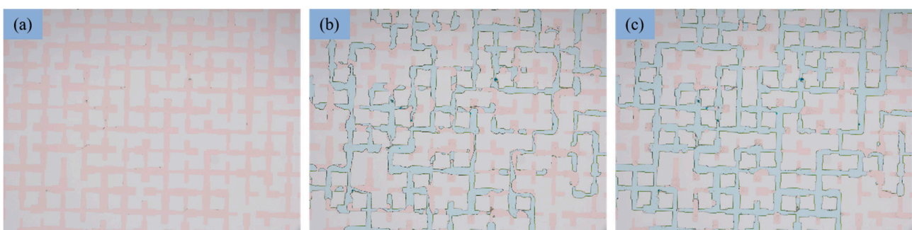
Figure 9. Visualization of oil–water distribution during micro-scale oil displacement (red represents oil and blue represents water). (a) Saturated oil, (b) primary water flooding, (c) secondary water flooding.
