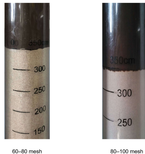
Figure 13. Penetration depth of sand bed of drilling fluid for strengthening plugging.
