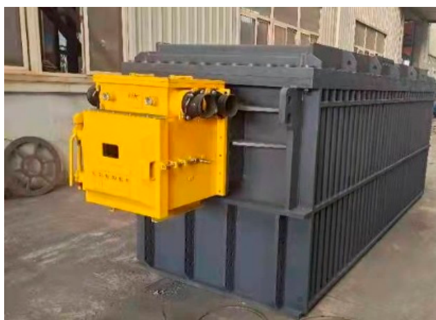
Figure 16. Overall Appearance of the Voltage Regulator.
