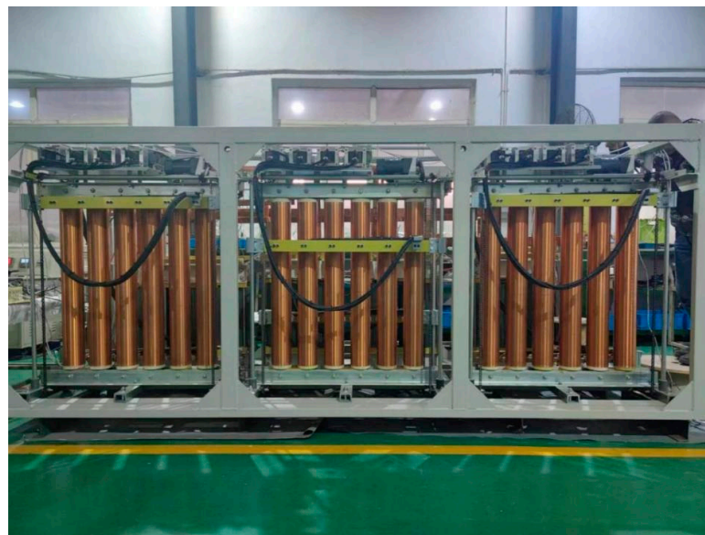
Figure 13. Physical Appearance of the Column-style Stepless Autotransformer.
