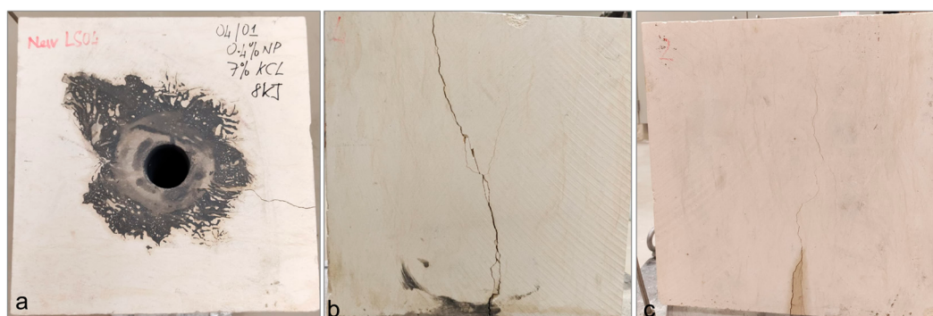
Figure 14. Prominent fracture development observed after NP-3PS on new Limestone LS03 under 8 kJ in 0.4 wt% NP + 7 wt% KCl + 0.18 wt% guar fluid: (a) Top view with marked date and parameters; (b,c) Side views of facet 4 and 2.
