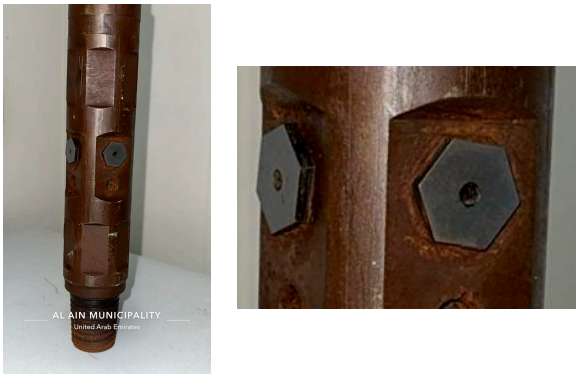
Figure 12. Abrasive jetting tool behavior after stimulation operation using QPQ 4145 material.
