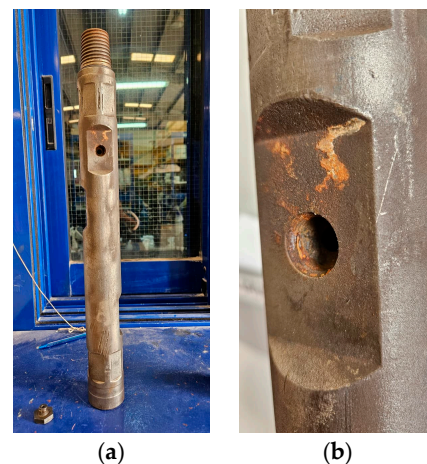
Figure 7. (a) Abrasive jet tool with lost jetting nozzle; (b) abrasive jet thread with pieces of 4140 material exposed at reservoir conditions.
