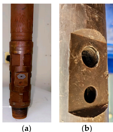
Figure 9. Abrasive jetting tool with 4145 materials implemented in the field. (a) Abrasive jet nozzle inspected after exposure to downhole conditions; (b) Zoomed view displaying jetting nozzle groove and intake thread without damage.
