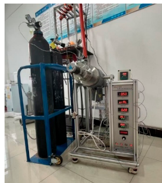
Figure 4. High-temperature high-pressure dynamic fluid loss apparatus.
