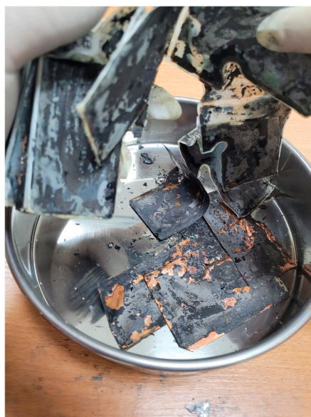
Figure 1. Disassembled cathode foils with LCO coating.
