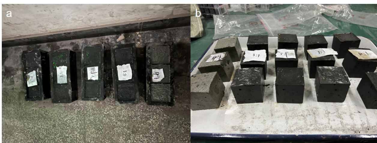
Figure 2. Test blocks: (a) prepared test blocks; (b) test blocks after de-molding.
