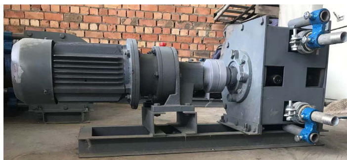
Figure 2. Physical image of the three-roller hose pump.
