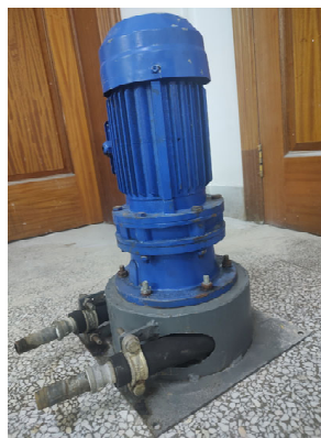
Figure 1. Physical image of the two-roller hose pump.
