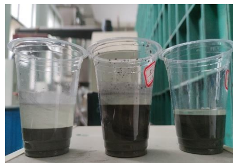
Figure 7. Severe dehydration of cement permeate samples.
