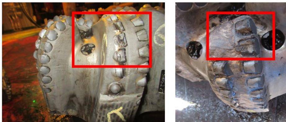
**Figure 10.** Field failure mode of PDC drill bits.
