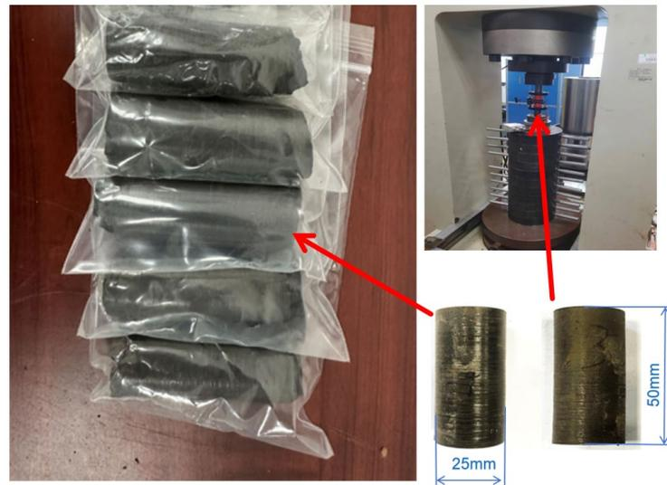
**Figure 1.** Uniaxial compressive strength test.
