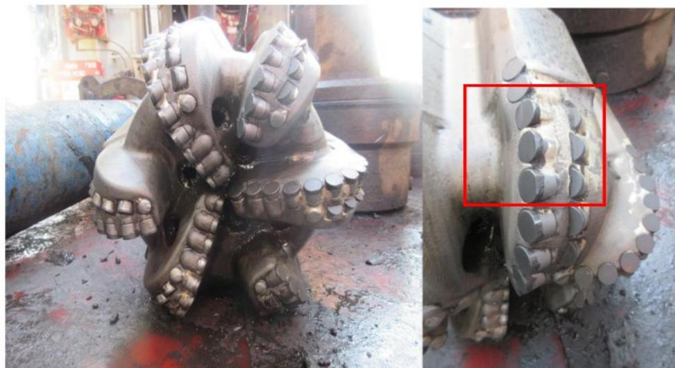
Figure 12. Appearance of the drill bit after optimization.
