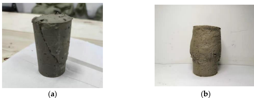
Figure 6. Failure modes of specimens under different confining pressures. (a) Low confining pressure; (b) high confining pressure.
