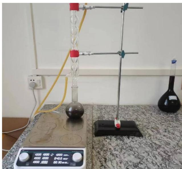
Figure 3. Experimental device for acid modification.
