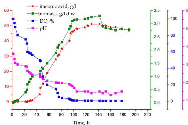
**Figure 3.** Evolution of parameters (itaconic acid, cells dry weight, dissolved oxygen, pH) during aerobic cultivation of *A. terreus*.
