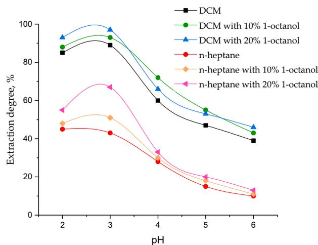
**Figure 6.** Influence of pH values of the aqueous phase on itaconic acid extraction degree in the presence of a phase modifier (TOA = 120 g/L).
