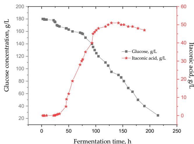
**Figure 2.** Glucose consumption and itaconic acid accumulation during *A. terreus* fermentation.
