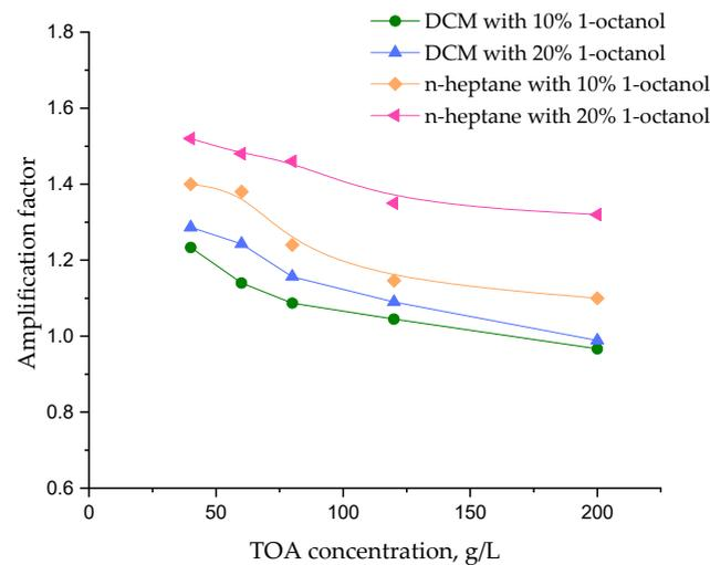
**Figure 9.** The variation of amplification factor with extractant concentration (pH of aqueous phase = 3).
