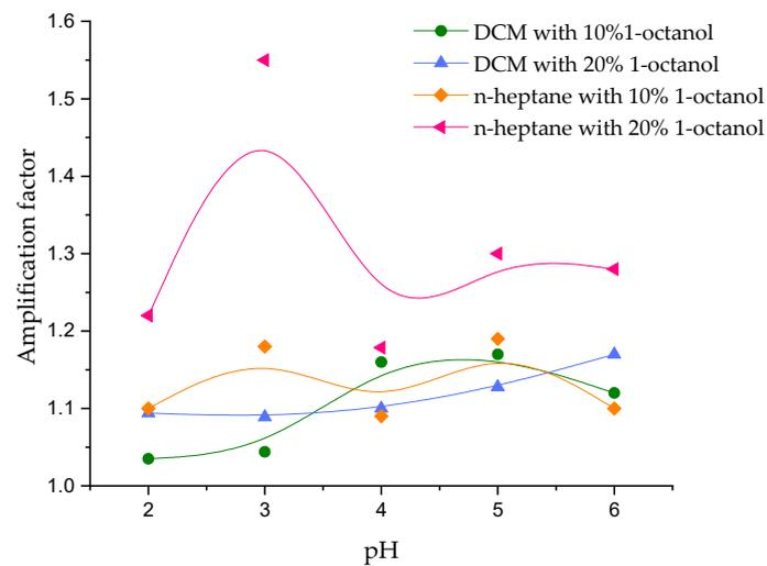
**Figure 8.** The variation of amplification factor with pH value of aqueous phase (TOA concentration = 120 g/L).
