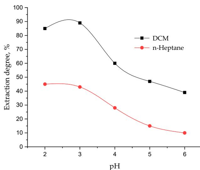
**Figure 4.** Influence of aqueous phase's pH value on itaconic acid extraction degree (extractant concentration, TOA = 120 g/L).
