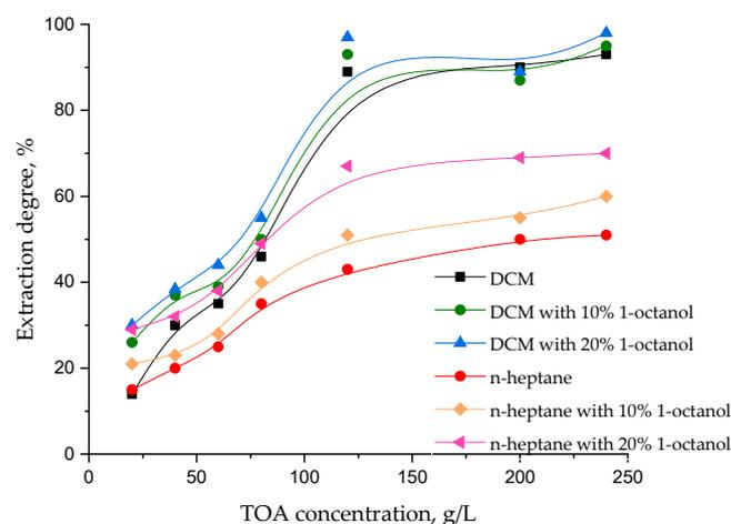
**Figure 7.** The influence of TOA concentration on the extraction degree of itaconic acid in the presence of phase modifier (aqueous phase's pH = 3).
