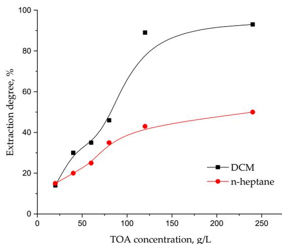
**Figure 5.** Influence of amine extractant concentration on itaconic acid extraction degree (aqueous phase pH = 3).
