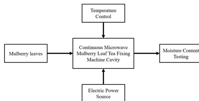
**Figure 6.** Overall framework of continuous microwave mulberry leaf tea fixation experiments.
