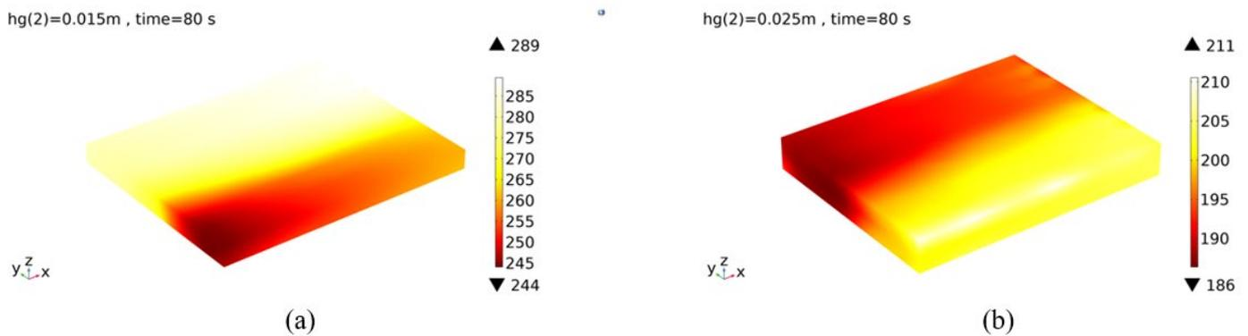
**Figure 14.** Temperature distribution after 80 s of blanching for various thicknesses. (a) The temperature distribution for a mulberry leaf thickness of  $hg = 0.015$  m and (b) the temperature distribution for a mulberry leaf thickness of  $hg = 0.025$  m.
