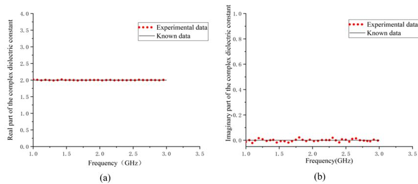
**Figure 4.** PTFE dielectric constant. (a) Relationship between real part and frequency; (b) Relationship between imaginary part and frequency.
