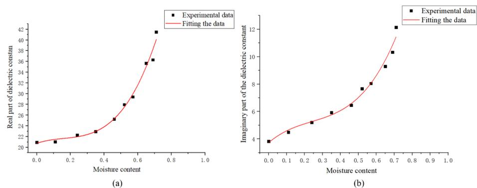
**Figure 5.** Dielectric properties of mulberry leaves. (a) Relationship between real part and moisture content; (b) Relationship between imaginary part and moisture content.
