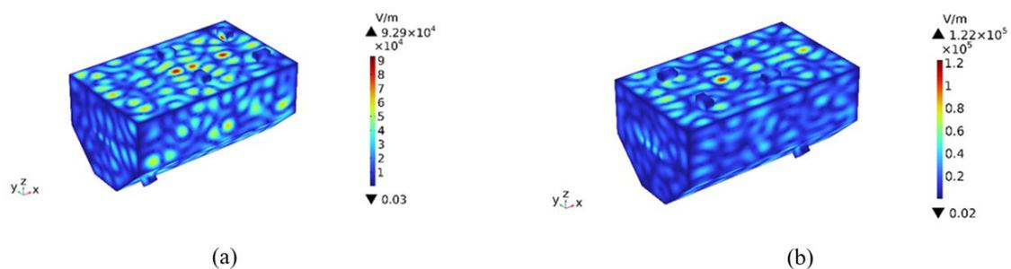
**Figure 11.** Electric fields at different port locations in the fixed machine cavity. (a) Electric field distribution of the first set of port parameters; (b) Electric field distribution of the seventh set of port parameters.
