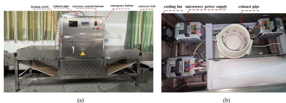
**Figure 7.** Physical system of continuous microwave fixer for mulberry leaf tea. (a) Continuous microwave mulberry leaf tea fixing machine; (b) Part of the power supply and cooling fan.
