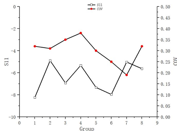
**Figure 13.** Impact of position variations on uniformity and S11 parameters.
