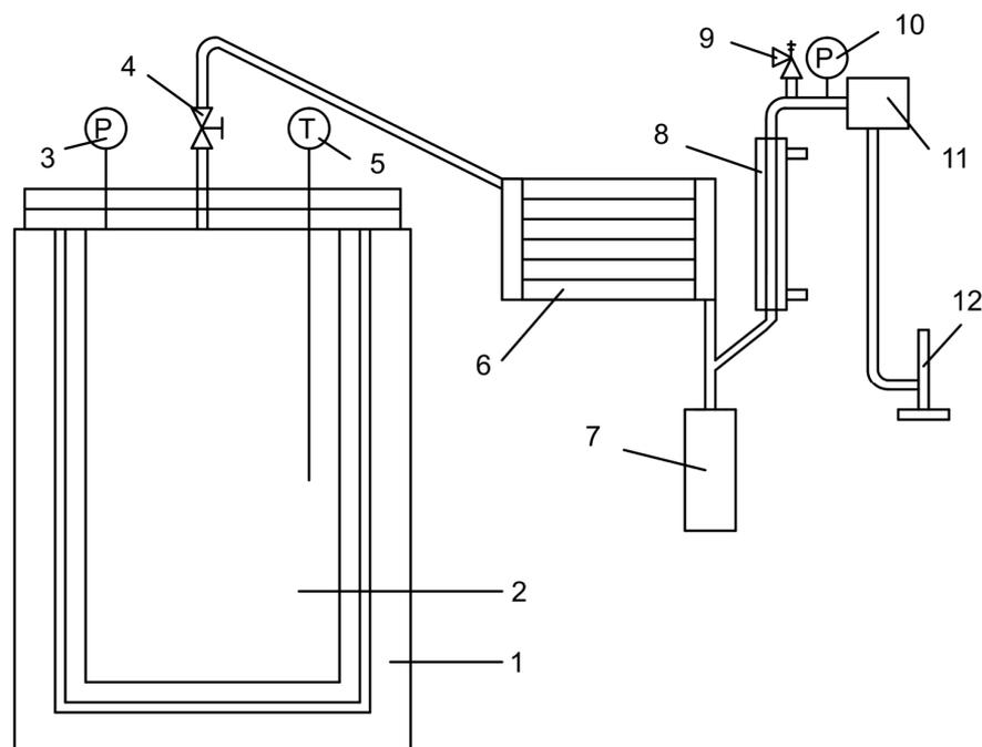
**Figure 1.** Slow pyrolysis system: 1—electric muffle furnace, 2—reactor, 3—pressure sensor, 4—thermocouple, 5—valve-pressure regulator, 6—air cooler-condenser, 7—liquid product collection container, 8—water cooler-condenser, 9—safety valves, 10—pressure sensor, 11—gas product volume measurement counter, 12—gas burner.
