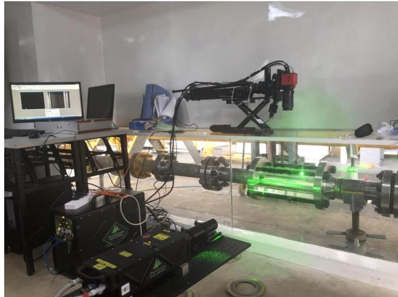
**Figure 12.** The PIV flowmeter for natural gas applications.
