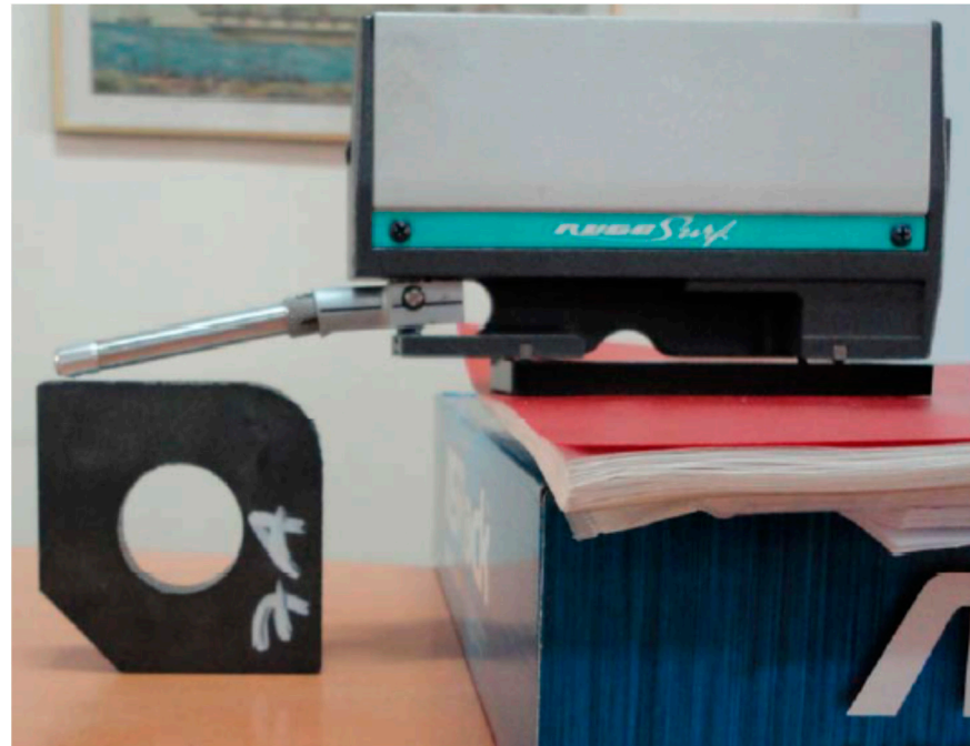
Figure 2. Surface roughness device and a completed cutting process unit.
