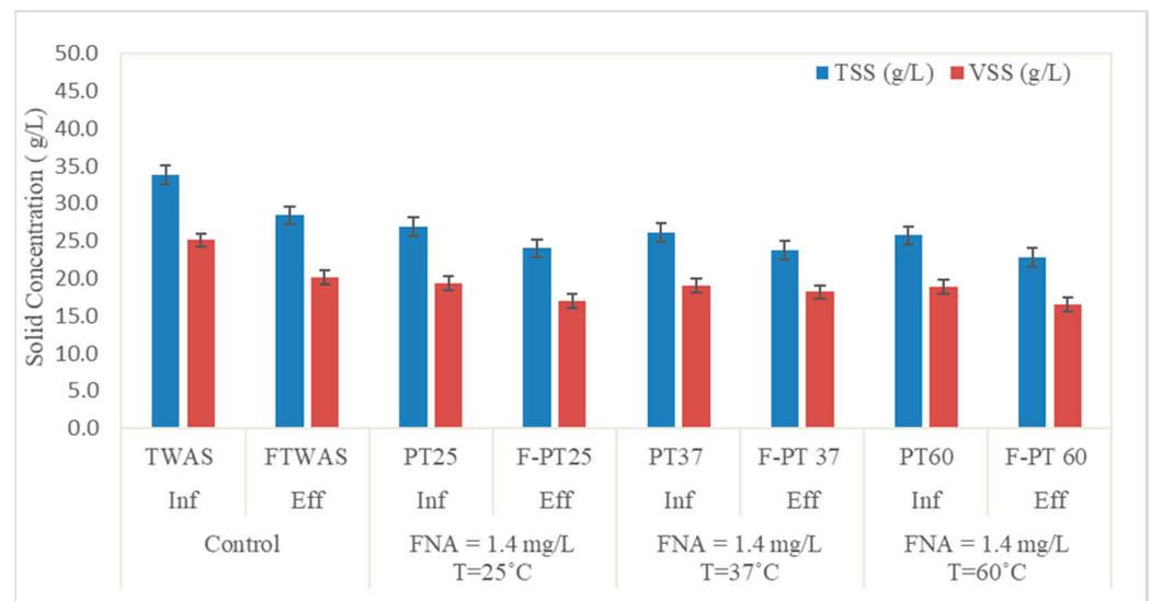
**Figure 3.** Concentration of the raw, pretreated, and fermented sludge; Combined FNA-heat pretreatment (error bars represent the standard errors).
