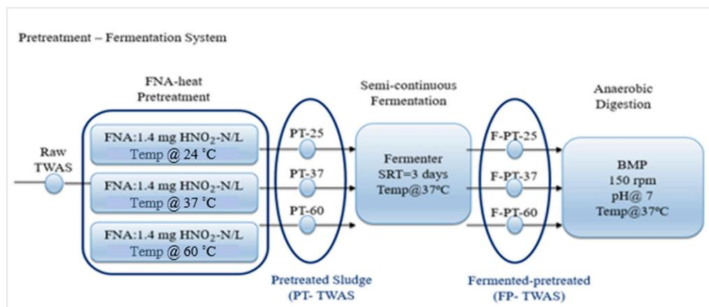
**Figure 2.** Experimental design of FNA-heat pretreatment and semi-continuous acidification/fermentation of control system.
