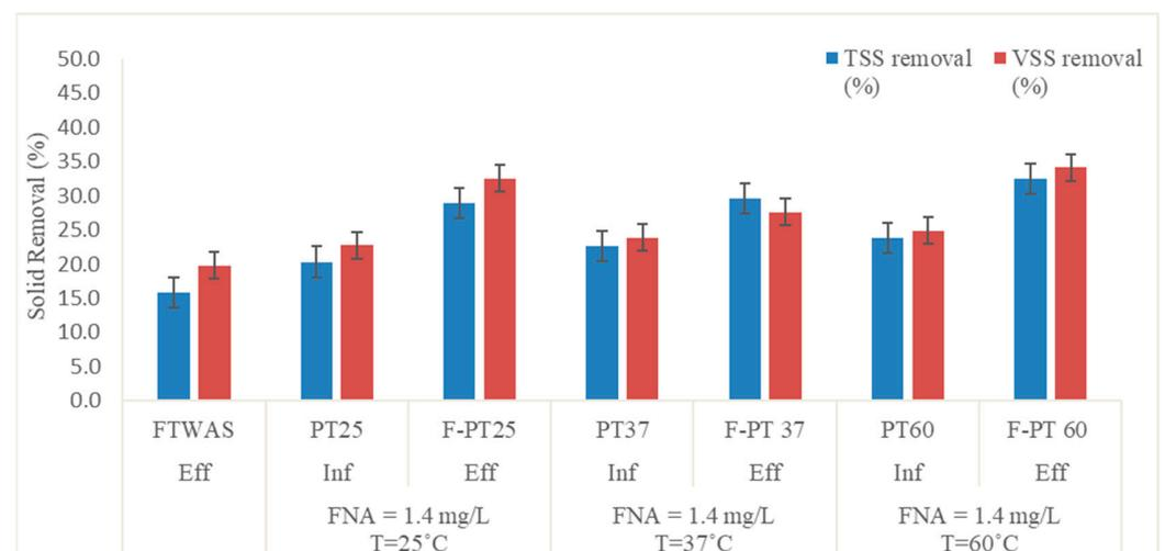
**Figure 4.** Percentage of suspended solids reduction via FNA-heat pretreatment, fermentation, and combined pretreatment/fermentation processes (error bars represent the standard errors).
