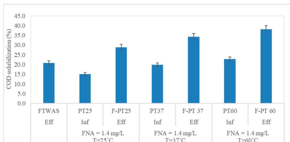
**Figure 6.** Degree of COD solubilization (%) in the fermented/FNA-heat pretreated samples compared to the raw TWAS (error bars represent the standard errors).
