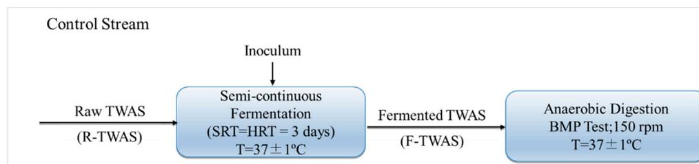
**Figure 1.** Experimental design of control system.
