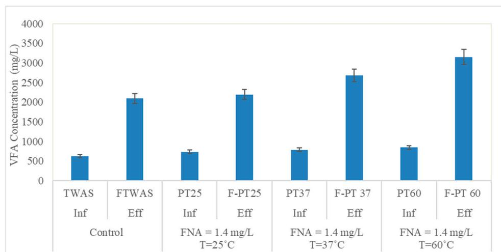
**Figure 7.** Total VFAs concentration (mg/L) in the fermented/FNA-Heat pretreated samples compared to the raw TWAS (error bars represent the standard errors).
