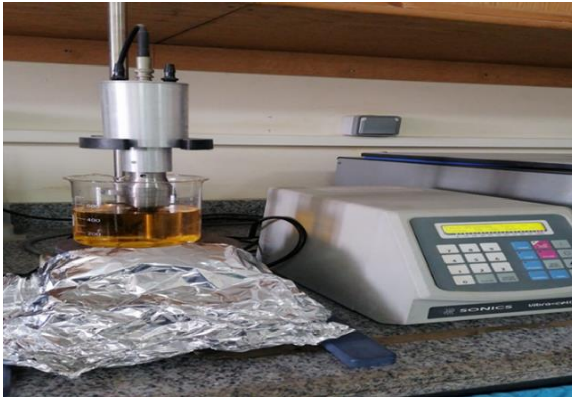
Figure 3. Preparation of nanofuels using the ultrasonicator.
