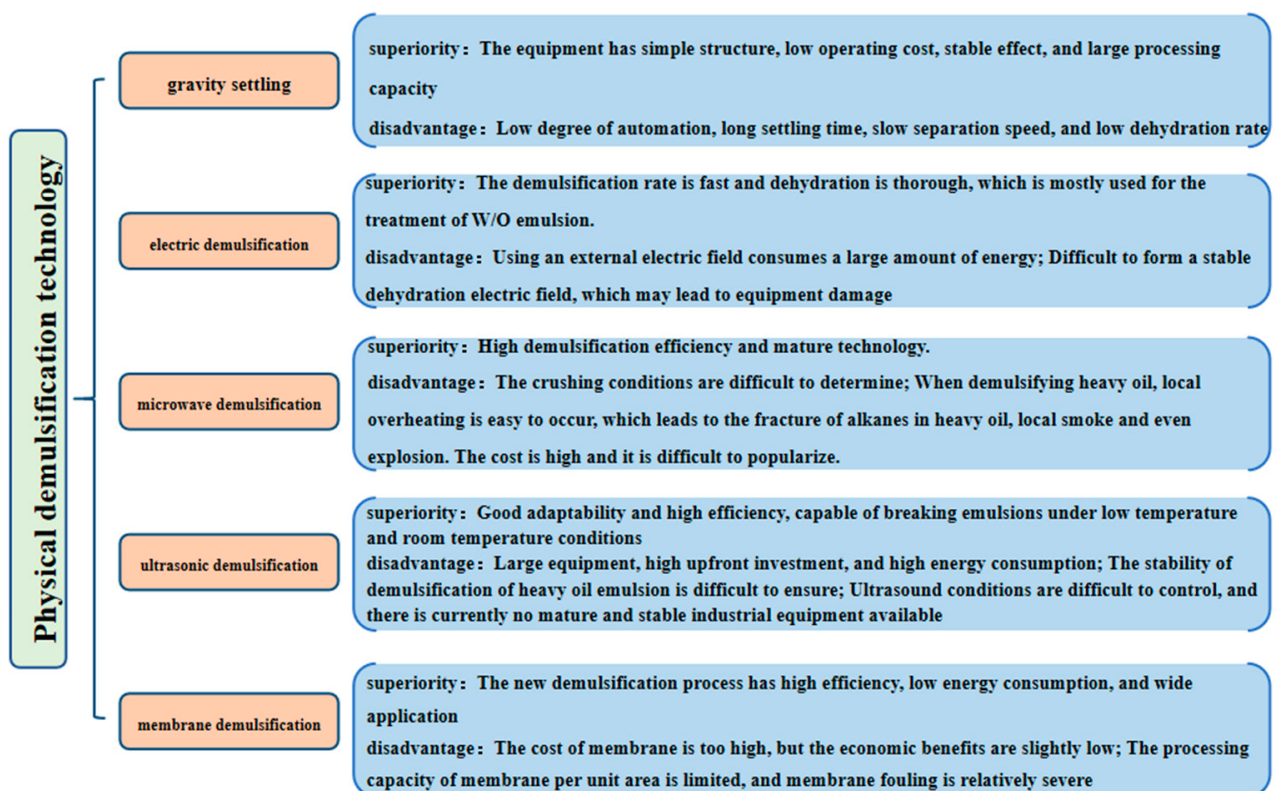
Figure 3. Comparison of physical demulsification methods for crude oil emulsions.
