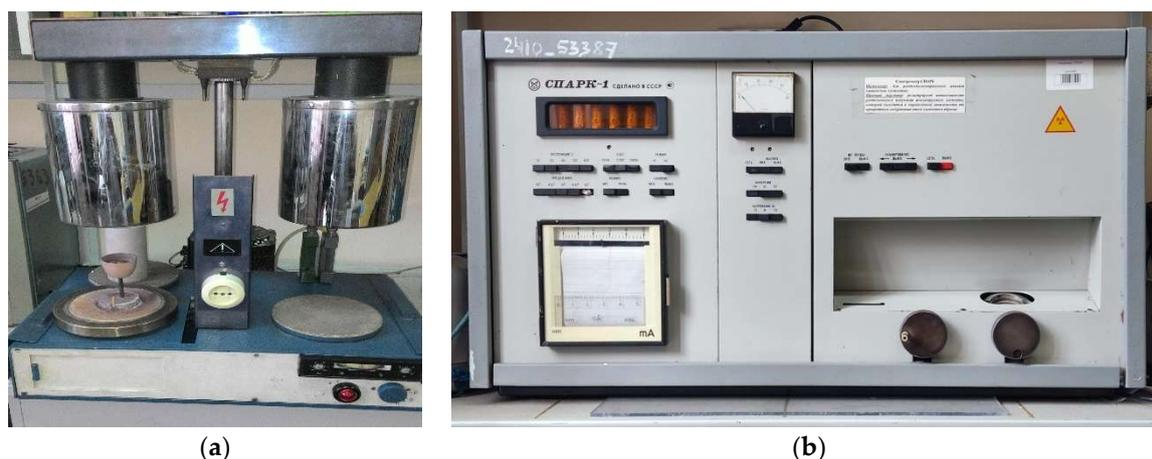
**Figure 2.** Firing unit with the IRT-2 temperature controller (a) and the SPARK-1 X-ray fluorescence analysis device (b).
