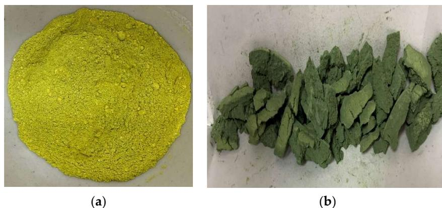
**Figure 8.** Photos of the samples of the tungstic acid (a) and the product after calcination (b).
