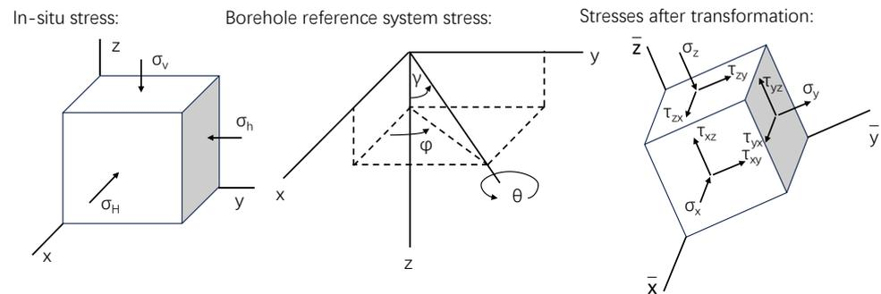
**Figure 1.** Transformation diagram of stress coordinates around a borehole.
