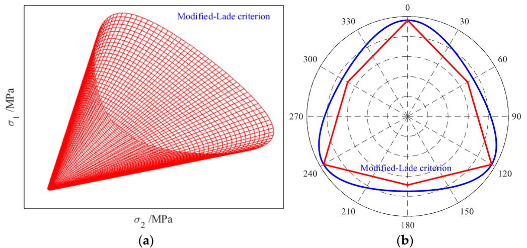
**Figure 2.** The failure envelopes the characteristics of the modified Lade criterion in the principal stress space and  $\pi$ -plane. (a) Yield surface in the principal stress space. (b) Yield curve in the  $\pi$ -plane (Blue line).
