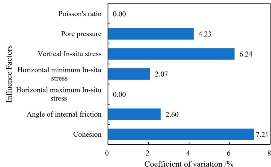
**Figure 5.** Sensitivity analysis of factors affecting borehole collapse for the horizontal well drilled in the direction of the maximum in situ stress.
