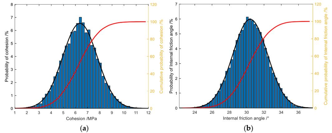
**Figure 3.** Distribution characteristics of input parameters: (a) cohesion and (b) internal friction angle.
