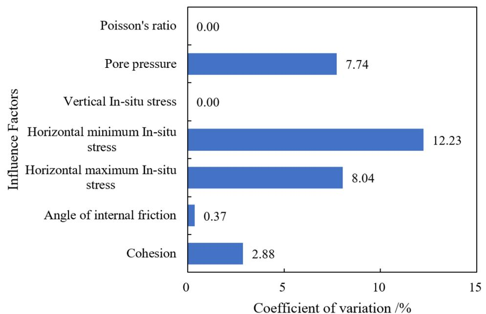
**Figure 6.** Sensitivity analysis of factors affecting vertical borehole breakout.
