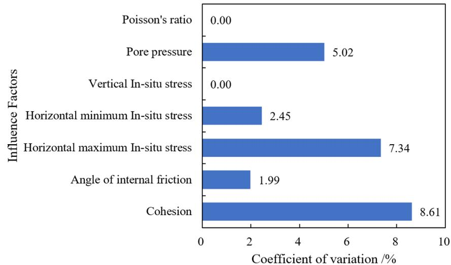
**Figure 4.** Sensitivity analysis of factors affecting vertical borehole collapse.
