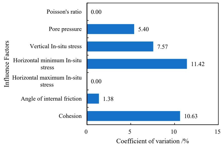
**Figure 7.** Sensitivity analysis of factors affecting borehole breakout for the horizontal well drilled in the direction of the maximum in situ stress.
