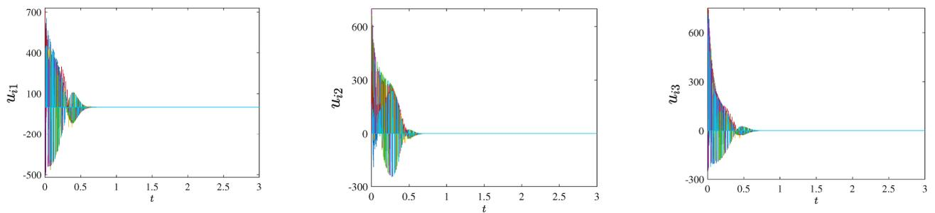
**Figure 8.** The update process of pinning controller  $u_i(t)$  with time ( $c_1 = c_2 = 0.1$ ).
