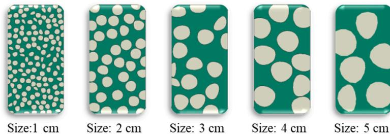
Figure 7. Schematic diagram of physical modeling of glutenite with different gravel sizes.
