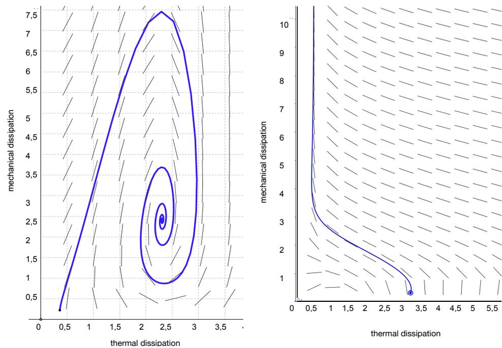
**Figure 11.** Interesting behavior of the energy dissipation rate for two selected mechanisms. (left) cyclic behavior as an indication of the possible formation of dissipative structures, (right) change in energy dissipation rate from thermal to mechanical dissipation.
