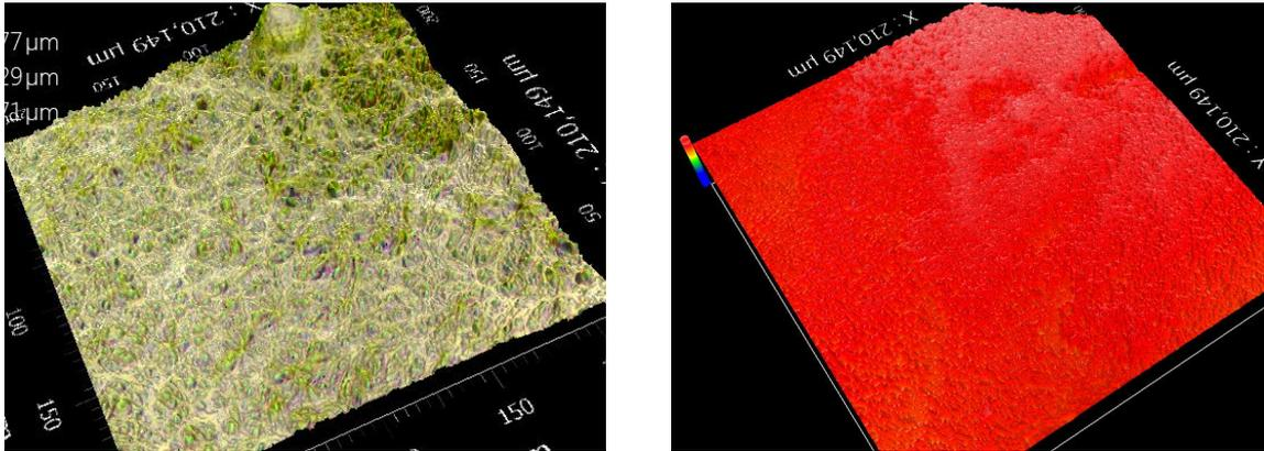
**Figure 7.** IFM-investigation (left) Li-sample unstressed, (right) Li-sample after stress.
