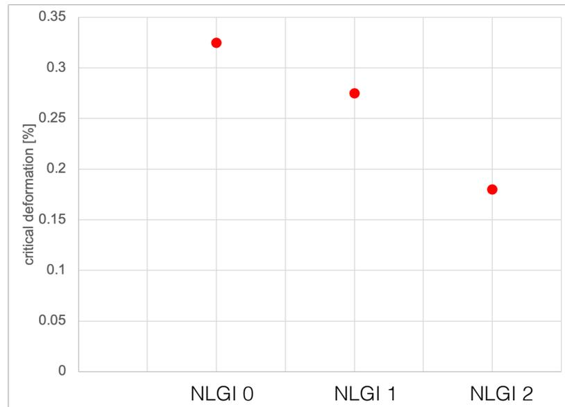
**Figure 10.** Decreasing critical deformation with increasing NLGI class (this corresponds to an increasing content of solids).
