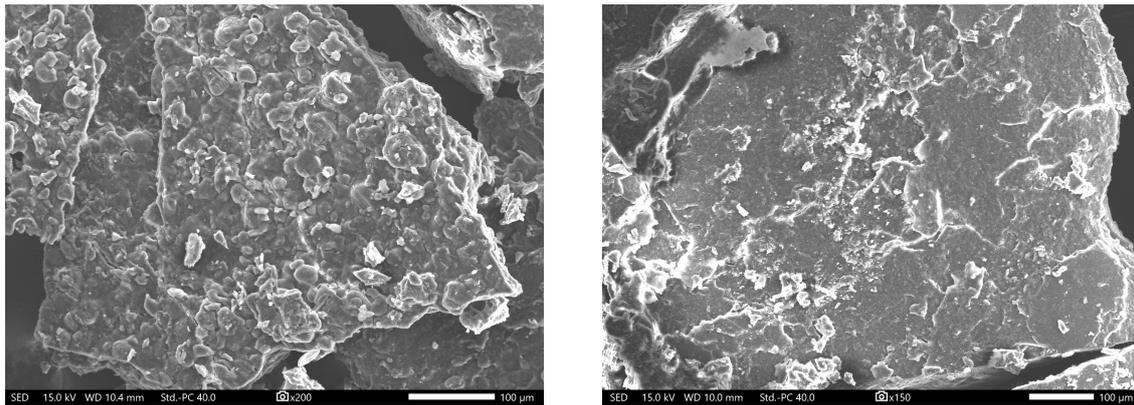
**Figure 4.** REM investigation of Ca-agglomerate (left) and an agglomerate from a polyurea sample (right).
