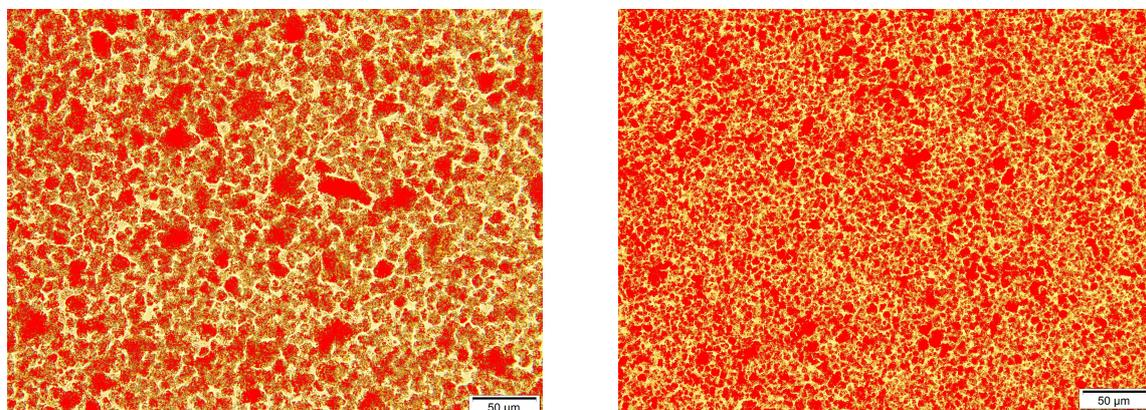
**Figure 6.** Transmitted light microscopy (left) grease sample before stress and (right) grease sample after stress.
