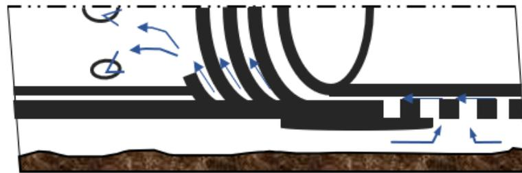
**Figure 1.** Schematic diagram of channel-type ICD.
