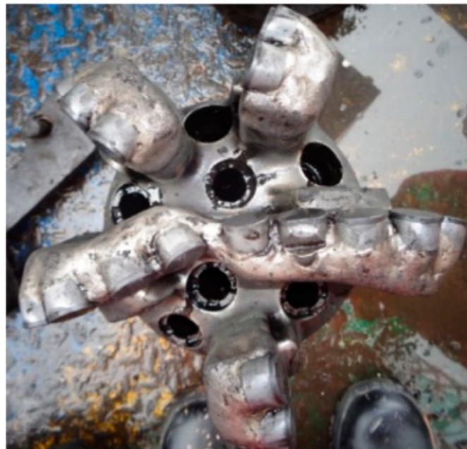
**Figure 8.** PDC bit after starting drilling.
