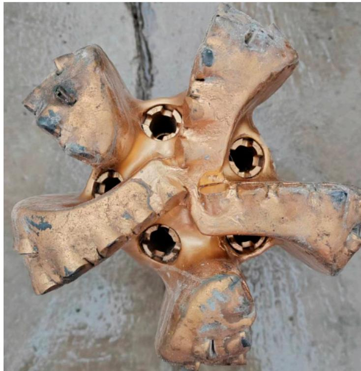
**Figure 10.** WS503HK PDC drill bit.
