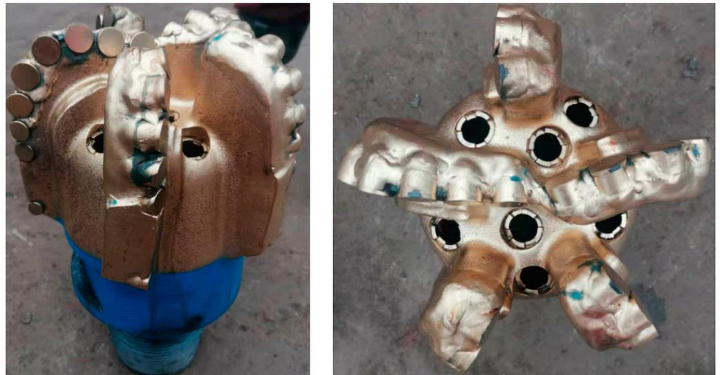
**Figure 7.** WS505HK PDC drill bit.
