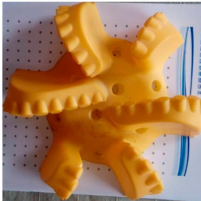
Figure 3. Mold of a carcass polycrystalline diamond compact (PDC) bit.
