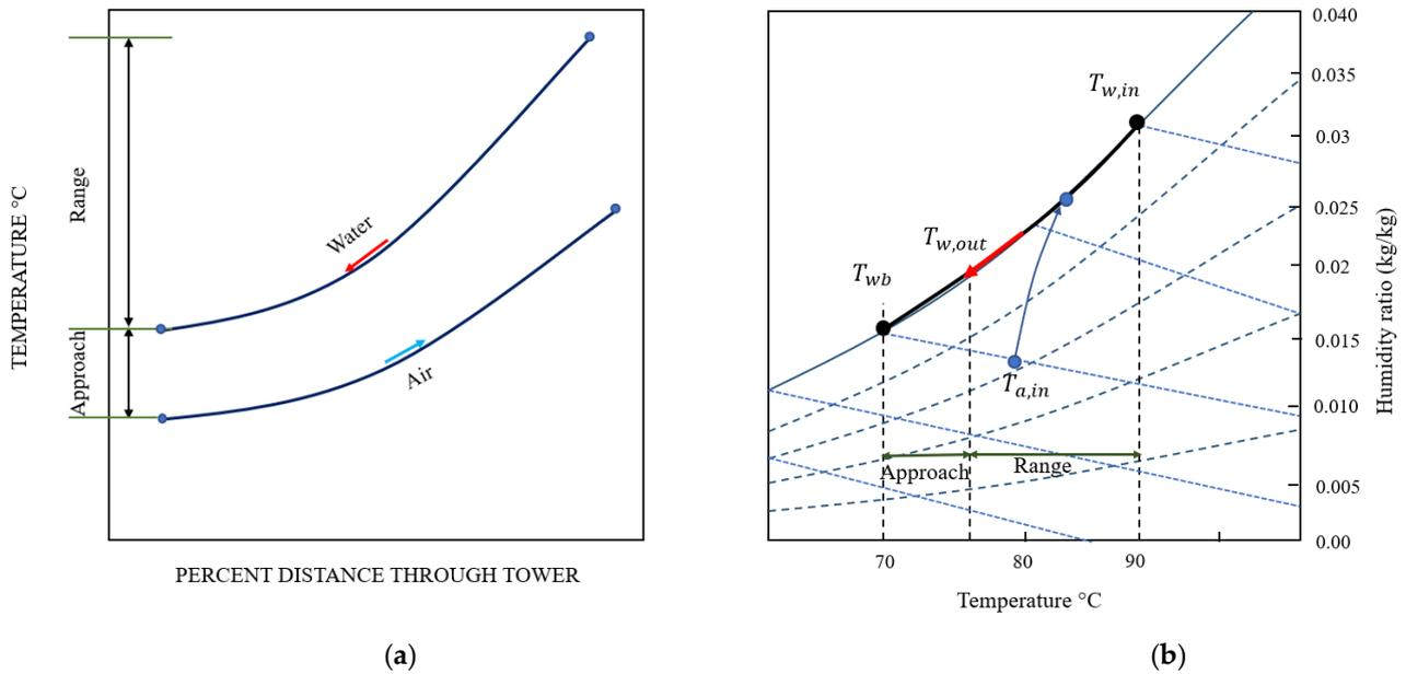
**Figure 7.** (a) Temperature relation between air and water and definition of Range and Approach; (b) psychrometric diagram for air passing through cooling tower.
