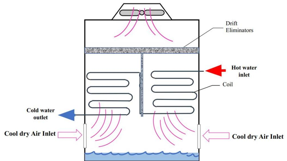
**Figure 4.** A schematic of a dry cooling tower.
