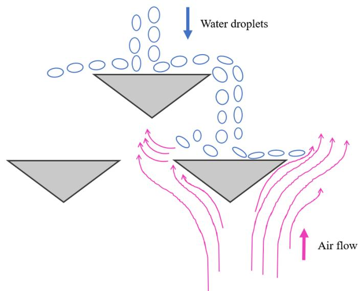
**Figure 5.** Triangular slat splash fill for cooling tower.
