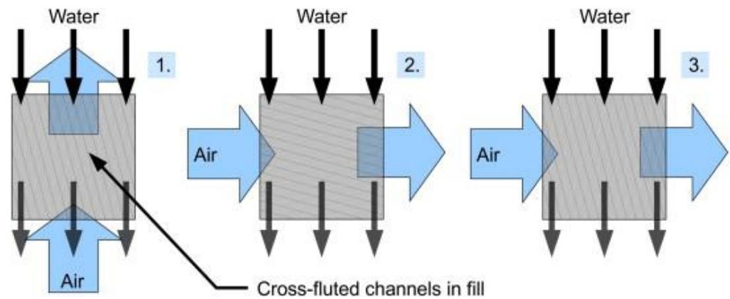
**Figure 8.** Three configurations of trickle fill: (1) counterflow with vertically oriented channels; (2) crossflow with horizontally oriented channels; (3) crossflow (counterflow config.) with vertically oriented channels [32].
