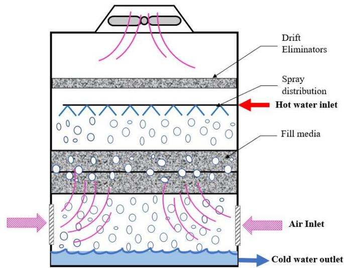
Figure 1. A schematic of direct-contact or open evaporative cooling tower.
