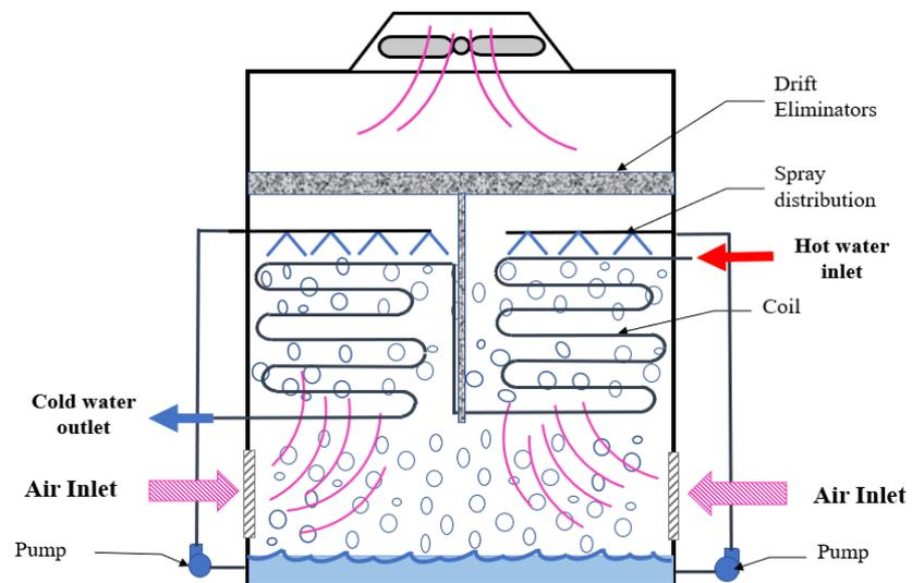
Figure 3. A schematic of wet cooling tower.
