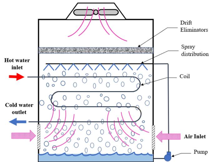
Figure 2. A schematic of indirect-contact or closed-circuit evaporative cooling towers.
