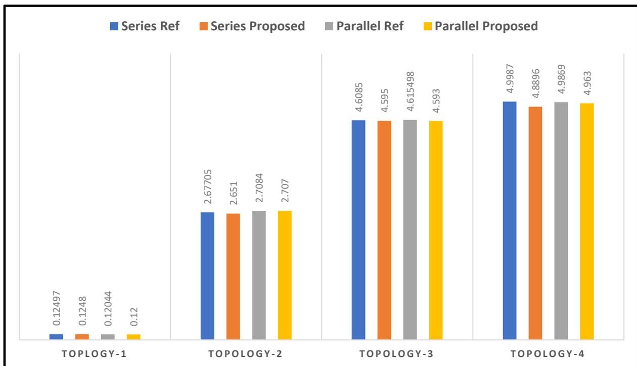
**Figure 3.** ITHD Comparison with proposed Filter.
