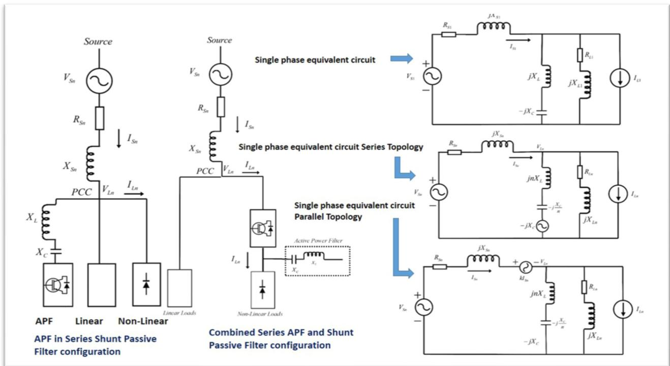
Figure 1. Filter topologies considered for parameter estimation.
