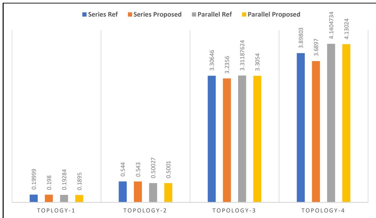
**Figure 4.** VTHD comparison with proposed filter.
