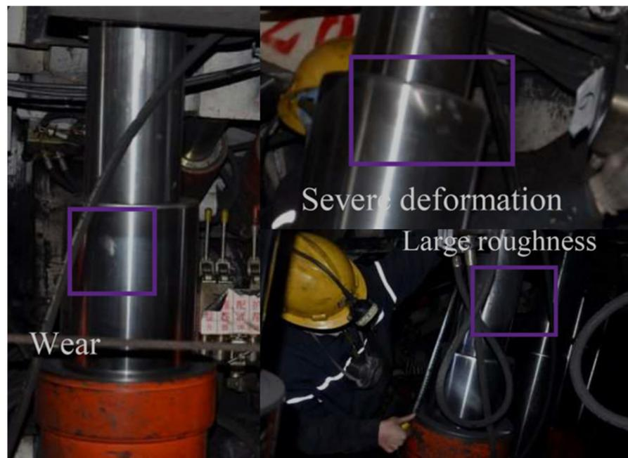
**Figure 2.** Rockfall impact damage to hydraulic support column.
