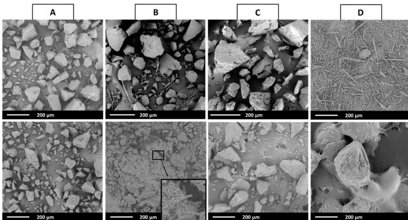
**Figure 11.** SEM images of samples before (**upper panel**) and after UV exposure (**lower panel**); (A) EUD, (B) physical mixture of VEN and EUD (1:5 *w/w*), (C) melt of VEN and EUD (1:5 *w/w*), (D) VEN.
