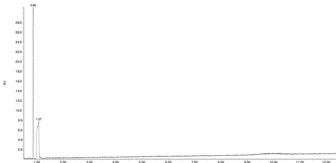
**Figure 9.** Chromatogram of the EUD after 78 days of exposure to UVA.
