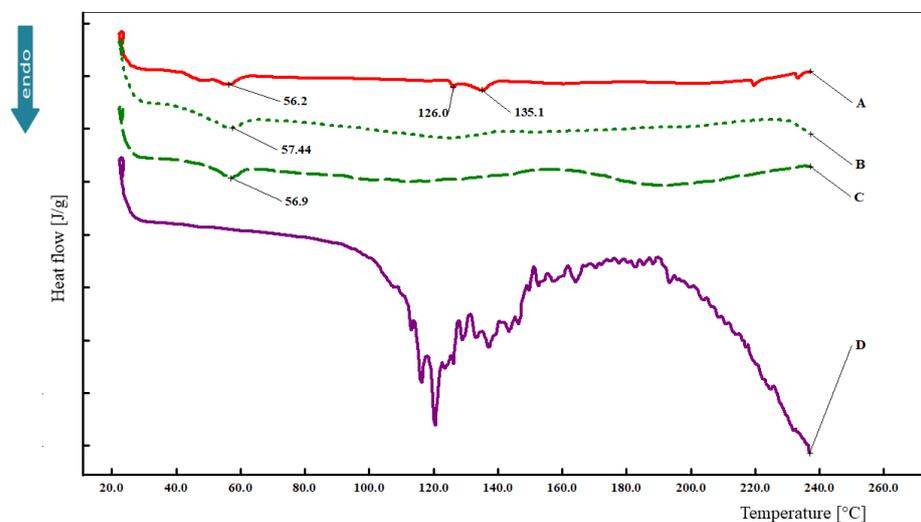
**Figure 13.** DSC curves of compounds under study after exposure to UVA: (A) EUD, (B) melt of VEN and EUD (1:5 *w/w*), (C) physical mixture of VEN and EUD (1:5 *w/w*), (D) raw VEN.
