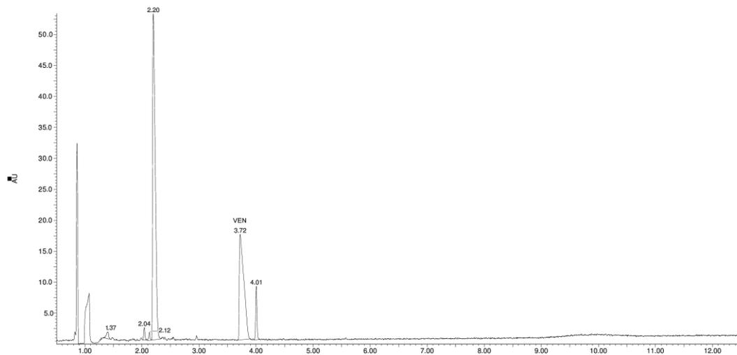
**Figure 5.** Chromatogram of the VEN—EUD physical mixture (1:5 *w/w*) after 64 days of exposure to UVA.
