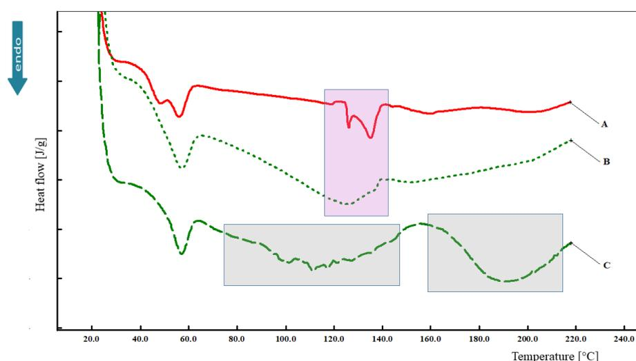
**Figure 14.** DSC curves of study compounds after exposure to UVA, shown using a different scale than in Figure 13: (A) EUD, (B) melt of VEN and EUD (1:5 *w/w*), (C) physical mixture of VEN and EUD (1:5 *w/w*).
