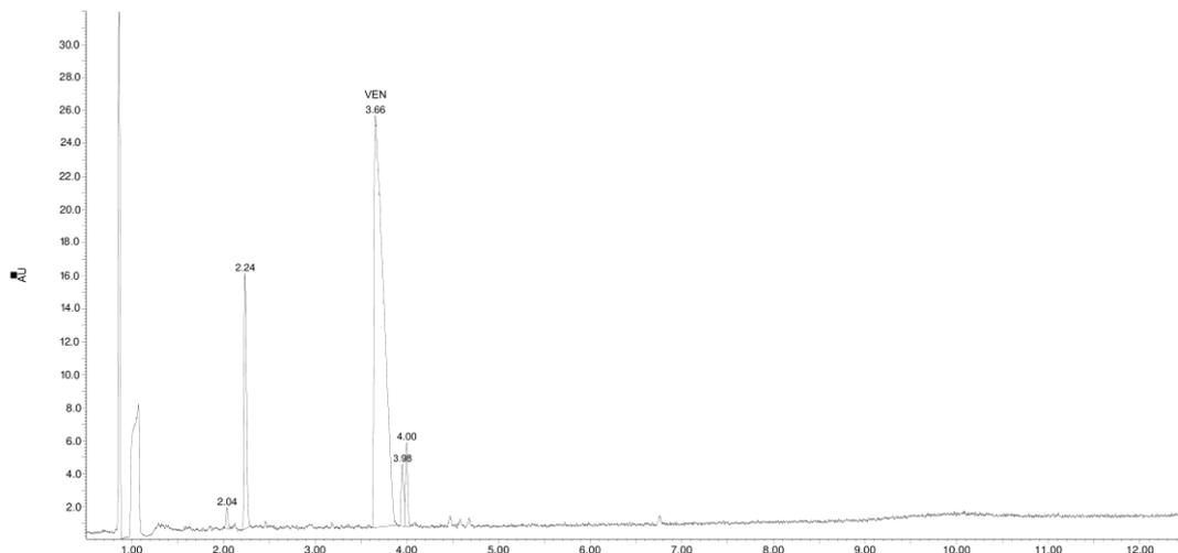
**Figure 6.** Chromatogram of the VEN—EUD melt (1:5 *w/w*) after 78 days of exposure to UVA.
