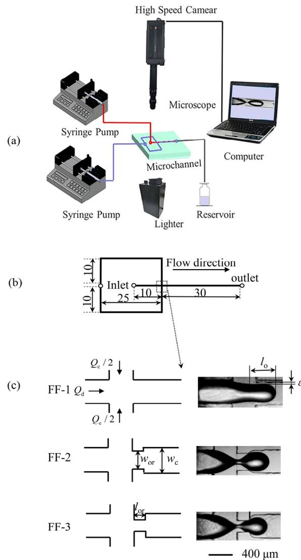
**Figure 1.** (a) Schematic diagram of the system for liquid–liquid two-phase flow. (b) Schematic diagram of microchannel. Unit: mm. (c) Left column: geometries of the channels near the cross junction (dashed line box in (b)). Right column: the two immiscible fluids meet at the cross junction of the microchannels.
