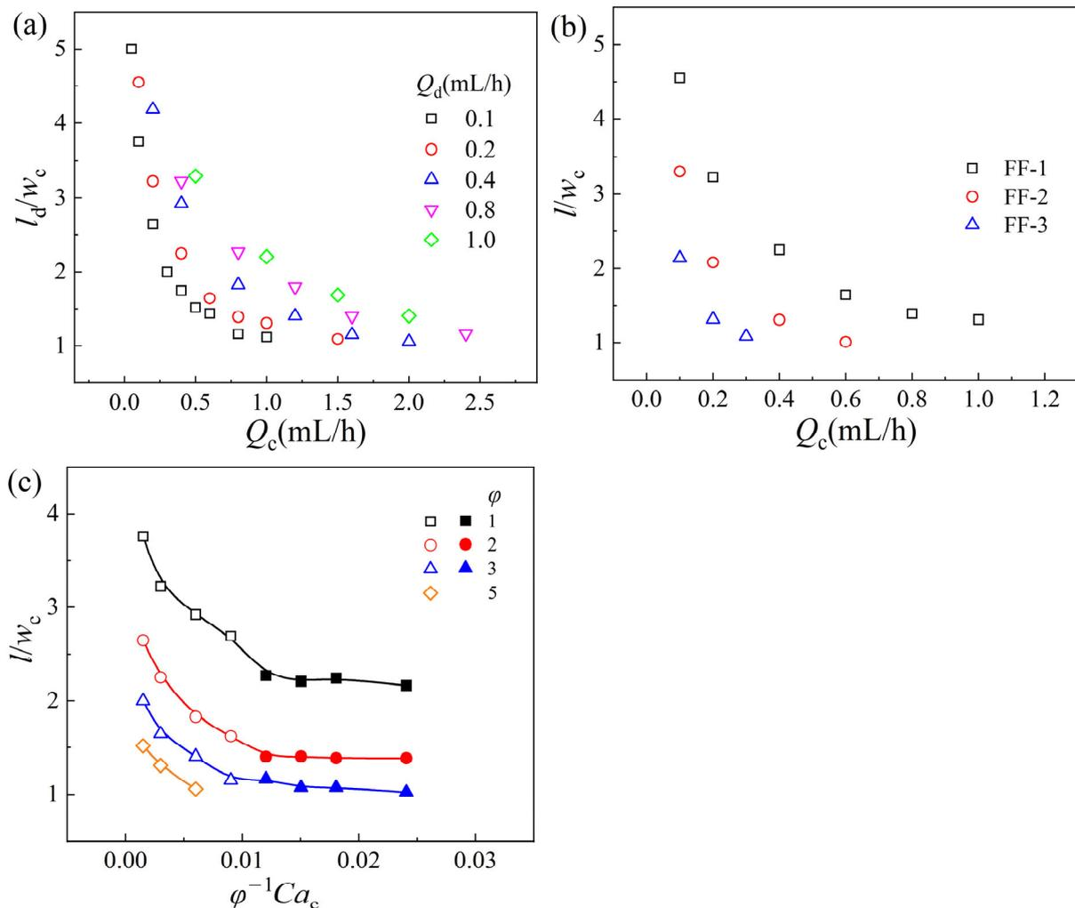
**Figure 5.** Effects of the operating conditions on the dimensionless droplet size  $l/w_c$ . (a) Effects of the flow rate of the continuous phase  $Q_c$  and the dispersed phase  $Q_d$  on  $l/w_c$  in FF-1. (b) Effects of the orifice size on  $l/w_c$ ;  $Q_d = 0.2$  mL/h. (c) Effects of the dimensionless number  $\varphi^{-1}Ca_c$  and  $\varphi$  on  $l/w_c$  in FF-1.
