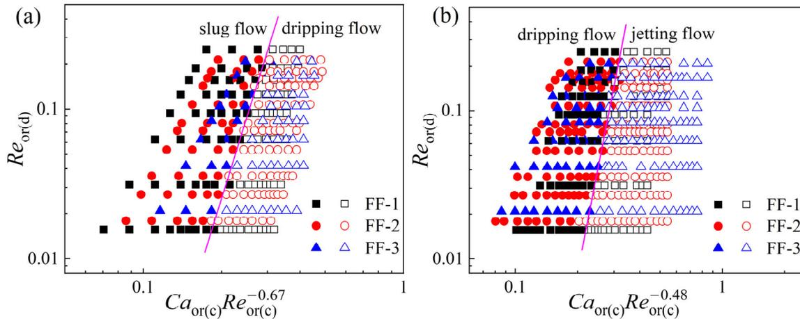
**Figure 4.** Proposed flow pattern maps and transition lines in microchannels with different orifice sizes. (a) Transition from slug flow to dripping flow; (b) transition from dripping flow to jetting flow.
