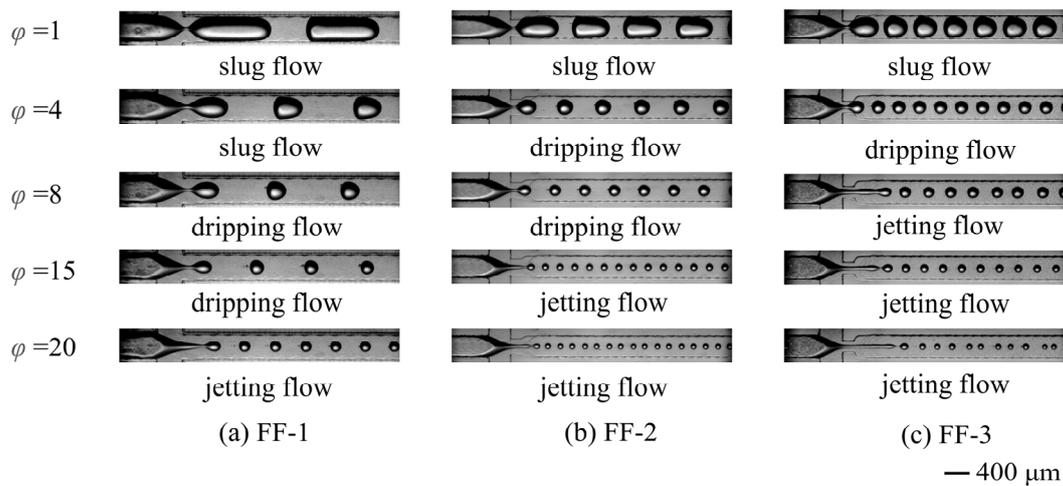
**Figure 2.** Liquid–liquid two-phase flow patterns in microchannels with different orifice sizes;  $Q_d = 0.4$  mL/h.
