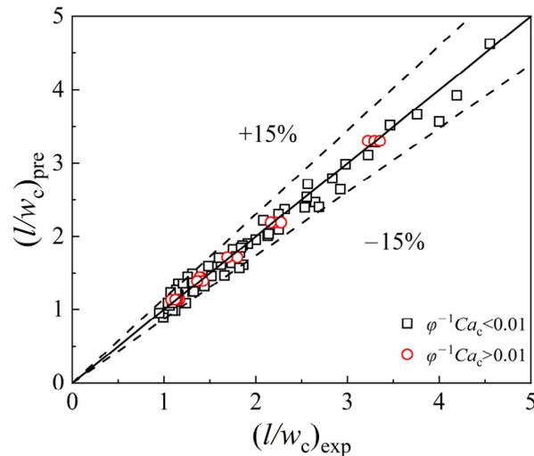
**Figure 7.** Comparison between calculated values  $(l/w_c)_{pre}$  of and experimental data  $(l/w_c)_{exp}$  on slug droplet size.
