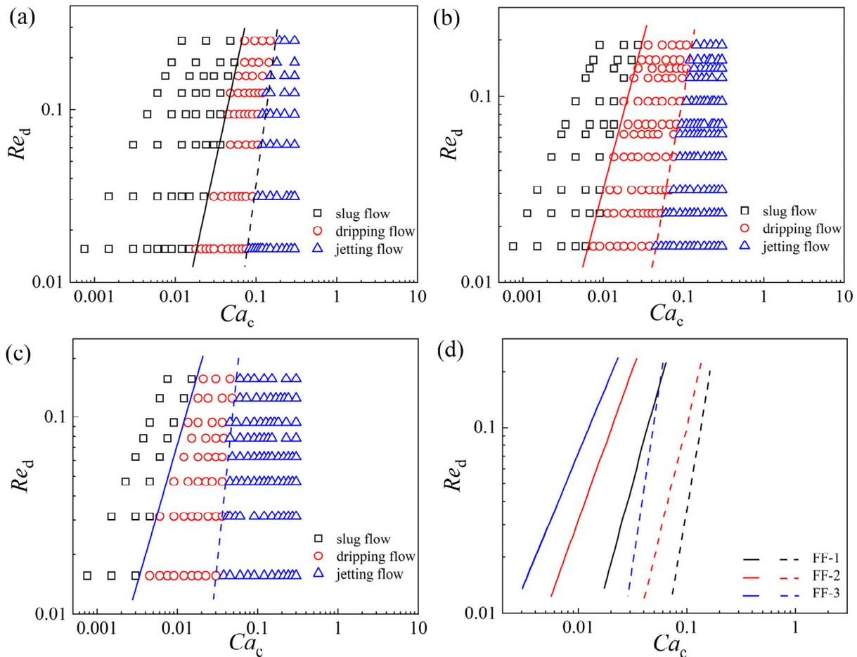
**Figure 3.** Flow pattern maps and transition lines of the adjacent flow pattern. (a) FF-1; (b) FF-2; (c) FF-3; (d) summary of transition lines of the adjacent flow pattern in three microchannels. Solid lines—transition lines from slug to dripping flow; dash lines—transition lines from dripping to jetting flow.
