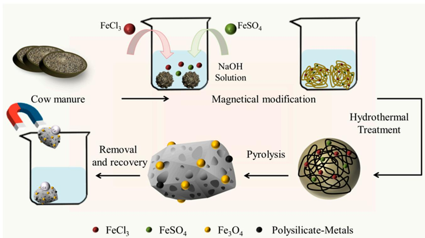
Figure 1. Preparation process for magnetic CM biochar.
