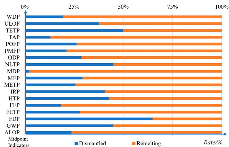
**Figure 7.** Comparison of the environmental impact of dismantling and remelting for the disposal of WPBs.
