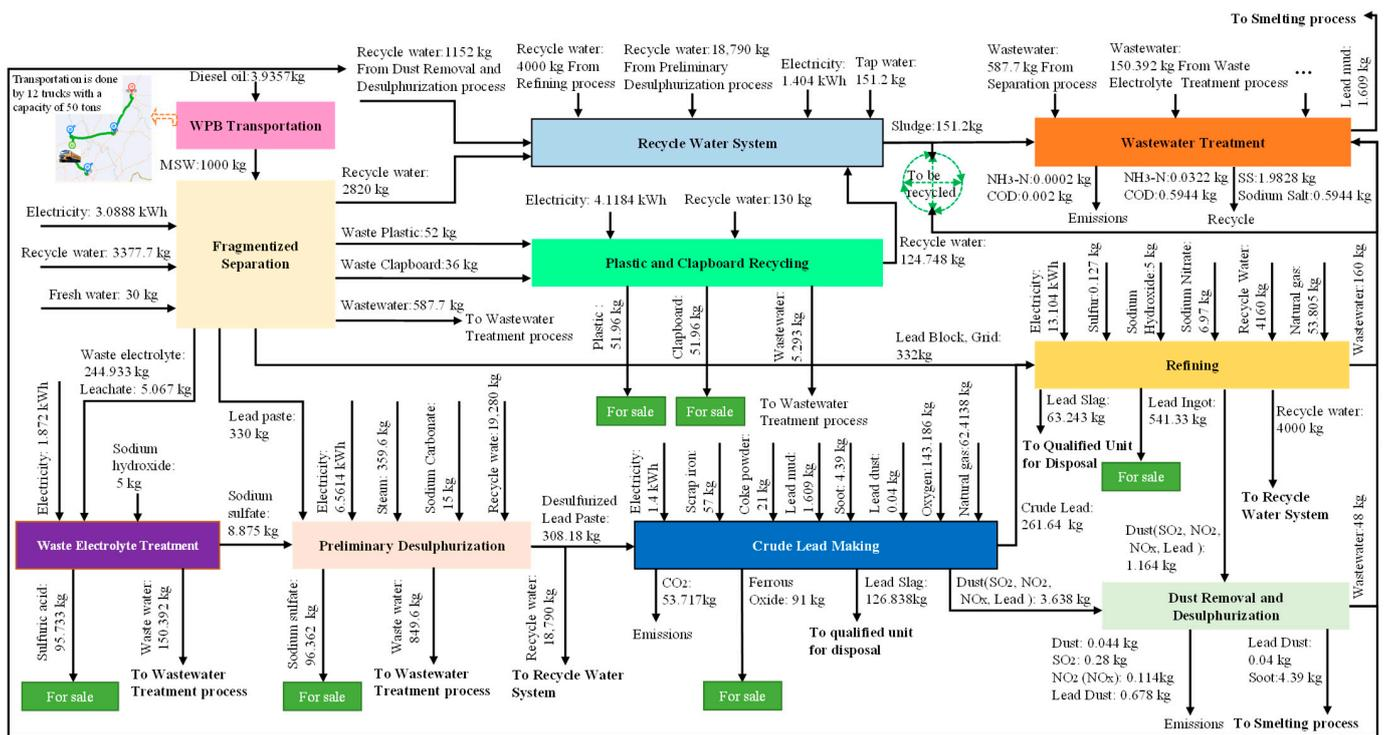
Figure 2. Quality and energy flows in one ton of WPB processing at the dismantling plant.
