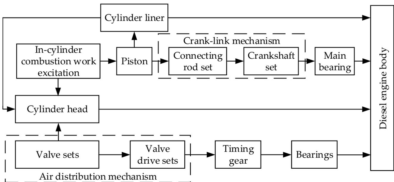
**Figure 3.** Diesel engine vibration excitation diagram.
