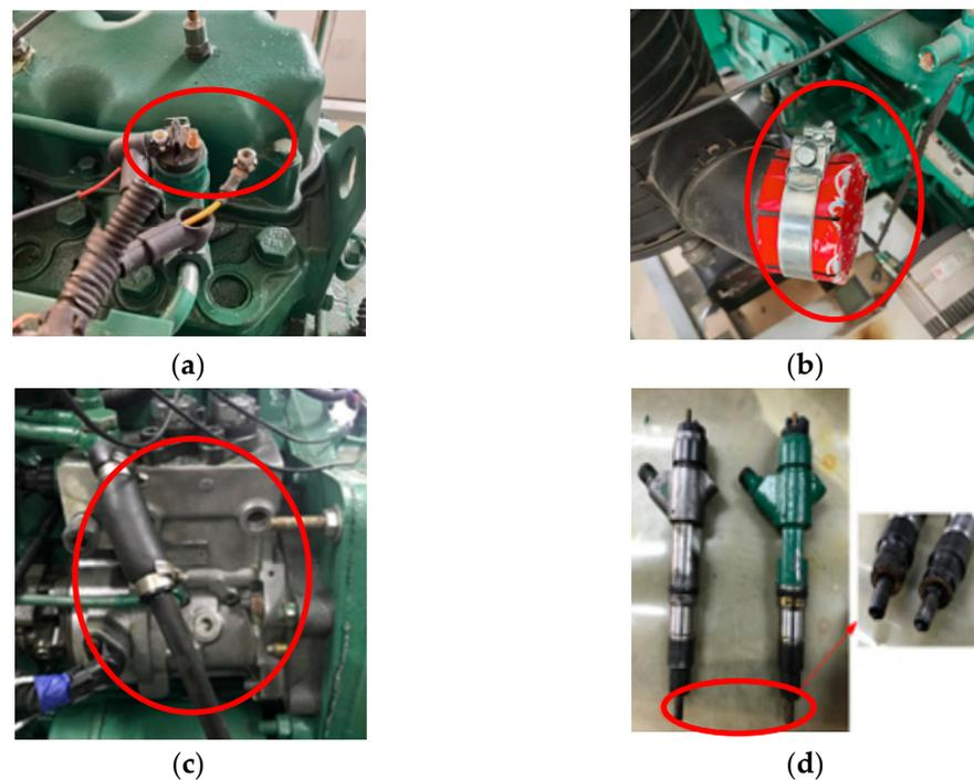
**Figure 6.** Diesel engine pre-set faults: (a) disconnect the ignition power cable; (b) add an air intake cover; (c) replace the faulty injection pump; and (d) replace the faulty injector.
