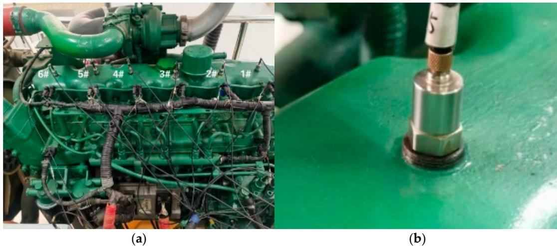
**Figure 4.** Mounting position of vibration sensors: (a) sensors mounting position and (b) diagram of sensors installation.
