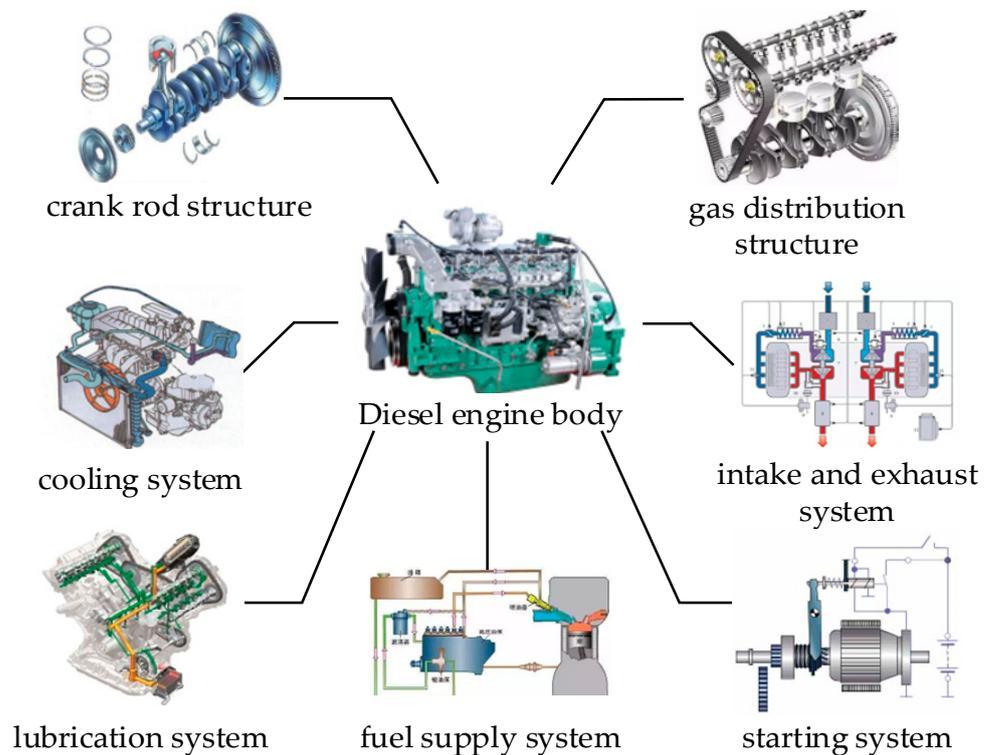
**Figure 1.** Schematic diagram of diesel engine components.
