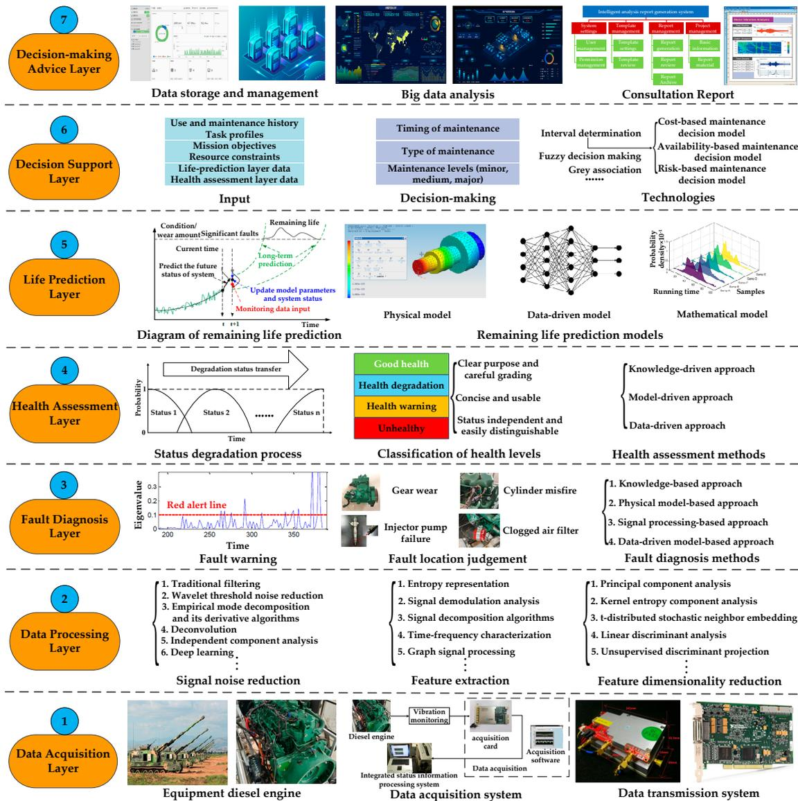
Figure 2. Diesel engine equipment—PHM system architecture.
