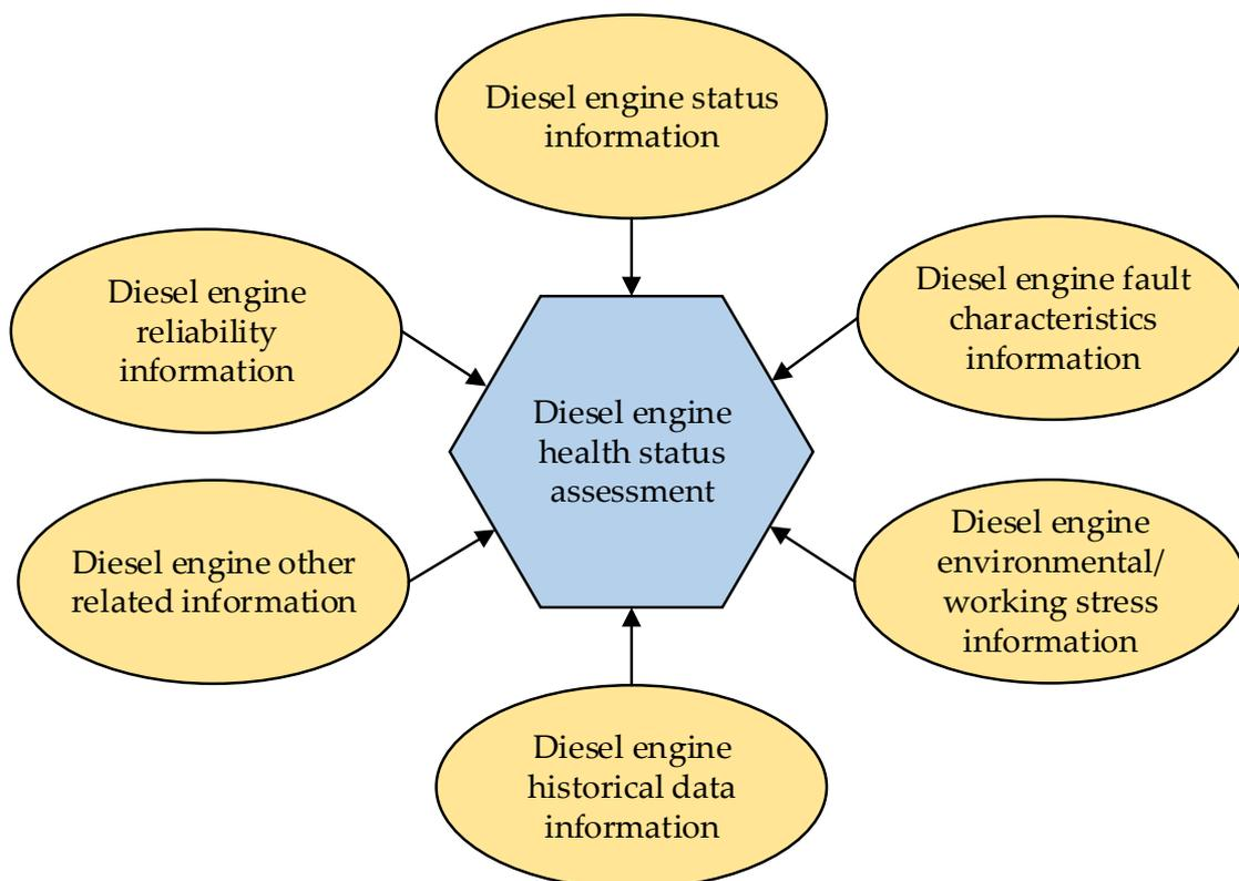
Figure 8. Multi-source characterization of diesel engine health status assessment.
