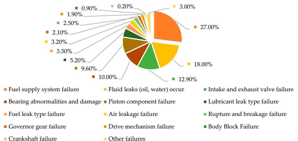
**Figure 5.** Statistical chart of diesel engine faults for a certain type of self-propelled artillery.
