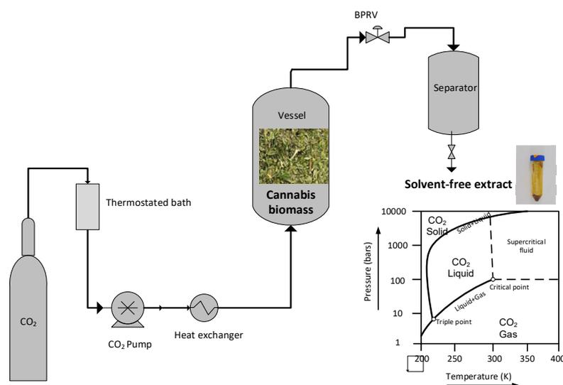
**Figure 1.** Supercritical carbon dioxide extraction unit.
