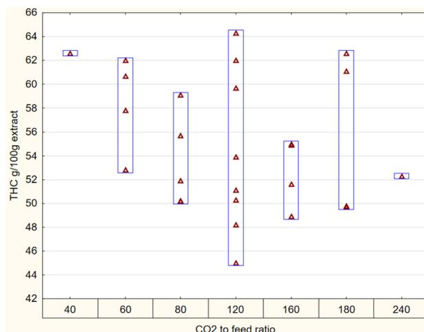
**Figure 4.**  $\Delta^9$ -THC as a function of CO<sub>2</sub>-to-feed ratio.
