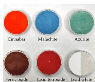
**Figure 3.** The color changes of mural blocks. (The left half area of each one is the control group; the right half area is irradiated at 20 kGy).
