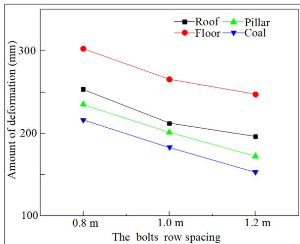
(a) Displacement graph of surrounding rock in the roadway with interlayer spacing of 10 m
