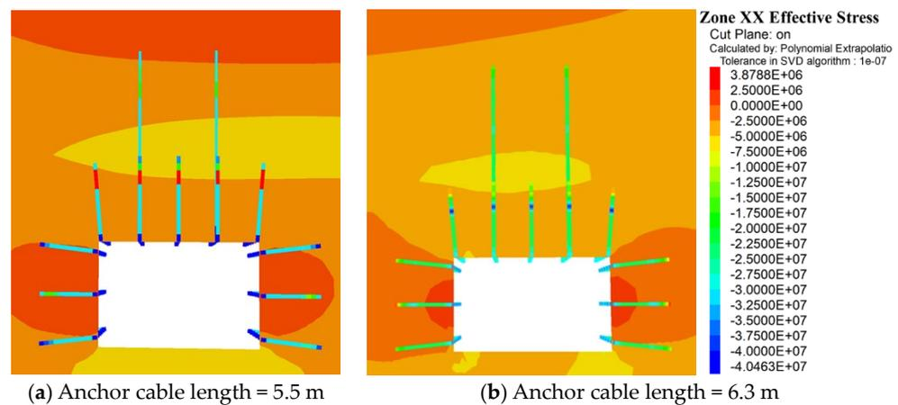
**Figure 15.** Stress contour map of the surrounding rock in the X-axis at different anchor cable lengths.
