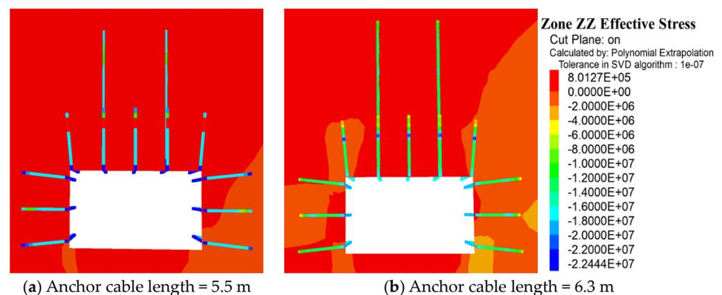
**Figure 16.** Stress contour map of the surrounding rock in the Z-axis at different anchor cable lengths.
