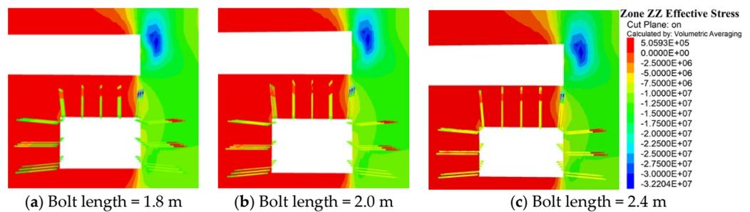
**Figure 13.** Stress contour map of the surrounding rock in the Z-axis at different bolt lengths.
