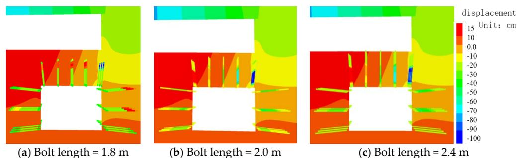
**Figure 14.** Distribution characteristics of the surrounding rock displacement at different bolt lengths.
