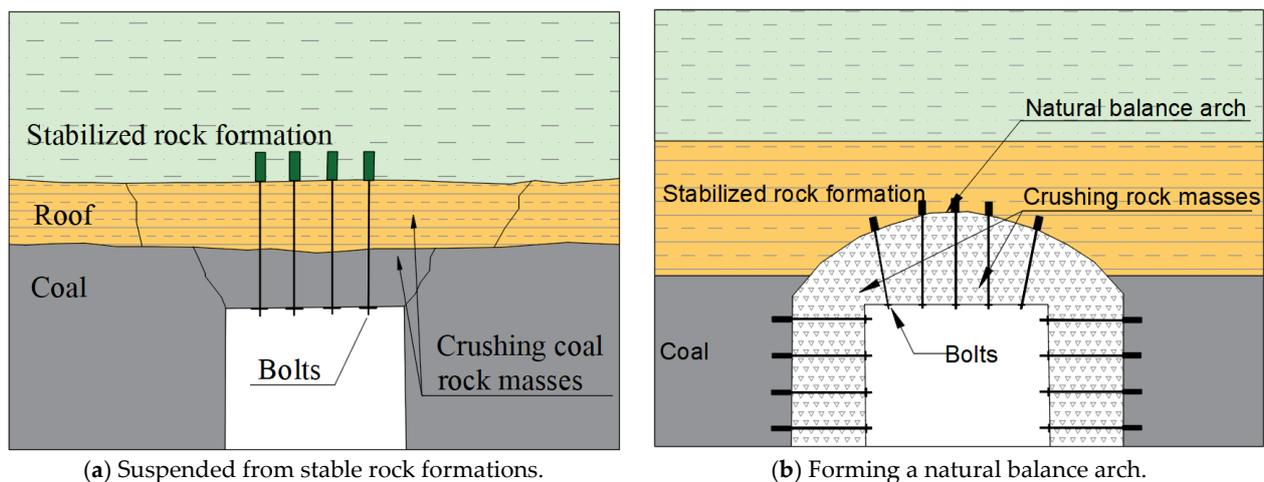
**Figure 1.** Bolt support suspension effect.
