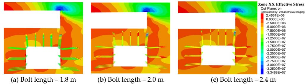
**Figure 12.** Stress contour map of the surrounding rock in the X-axis at different bolt lengths.
