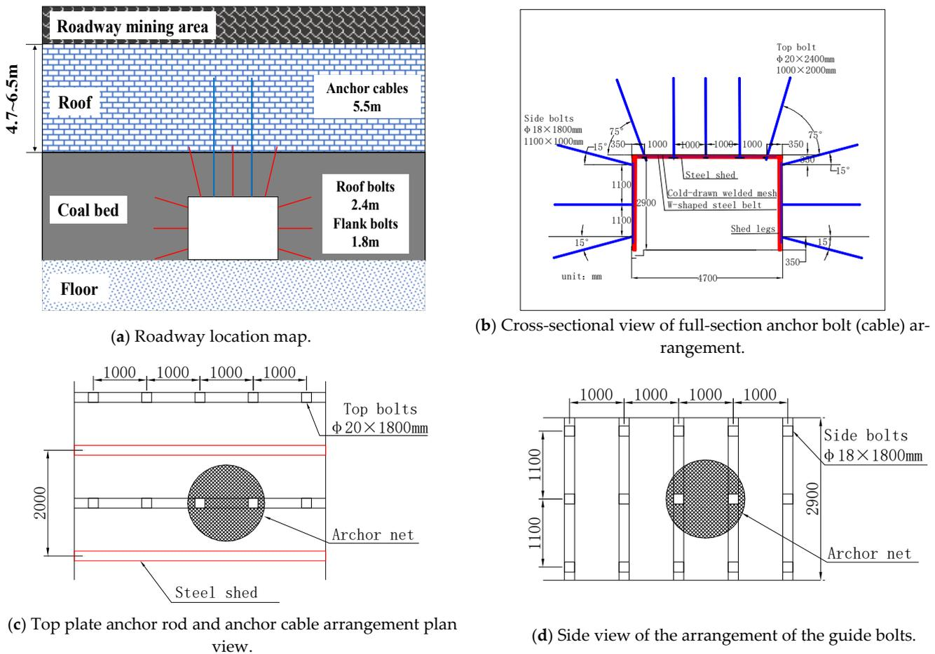
Figure 19. Support form for layer spacing of 2.5 m to 4.7 m: (a–d).
