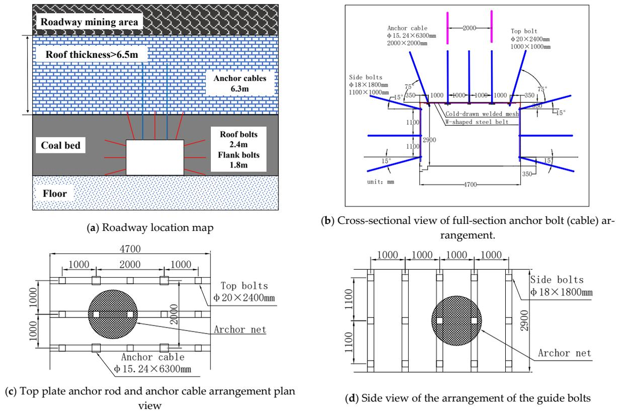
Figure 17. Support form for layer spacing greater than 6.5 m: (a–d).
