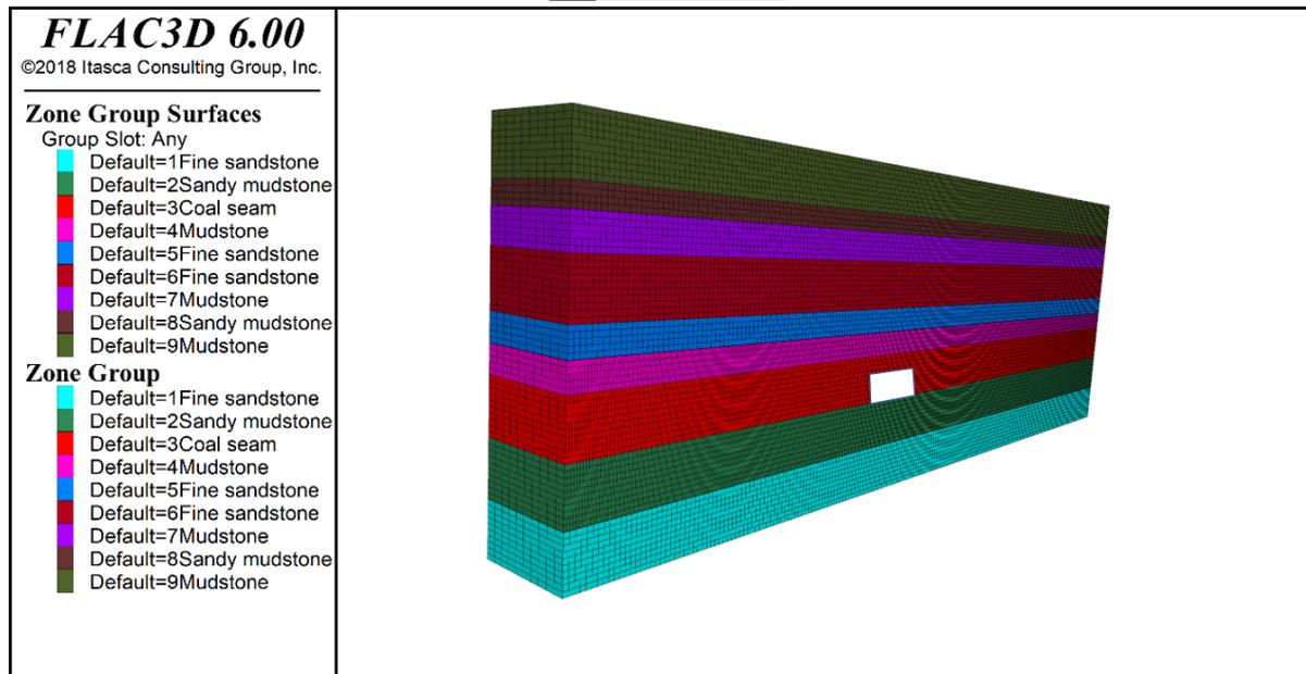
**Figure 7.** Numerical block model for simulation.
