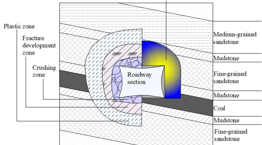
**Figure 2.** Model diagram of the loosening and anchoring composite bearing body of the surrounding rock.
