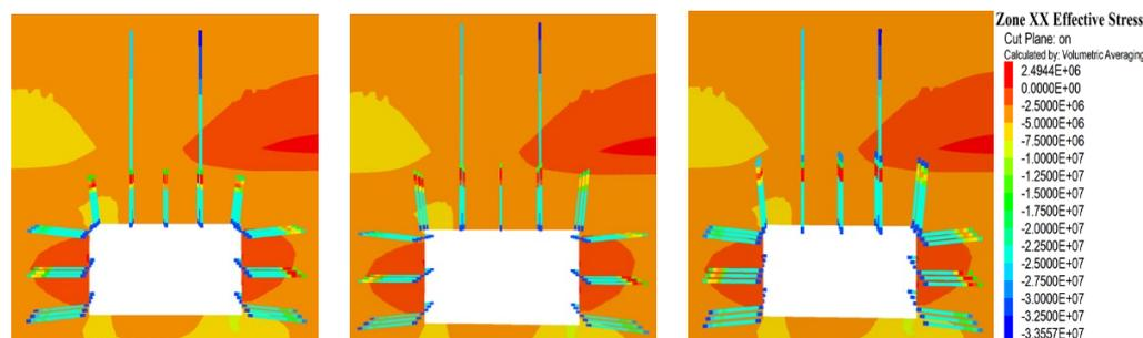
**Figure 9.** Stress contour map of the surrounding rock in the X-axis direction at different bolt lengths.
