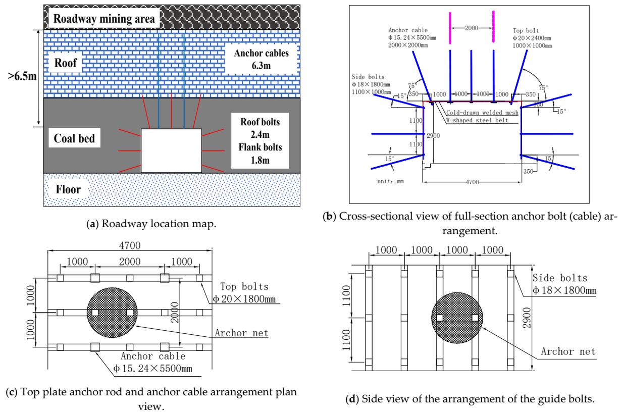
Figure 18. Support form for layer spacing of 4.7 to 6.5 m: (a–d).
