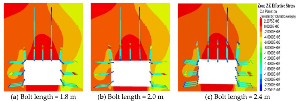
**Figure 10.** Stress contour map of the surrounding rock in the Z-axis direction at different bolt lengths.
