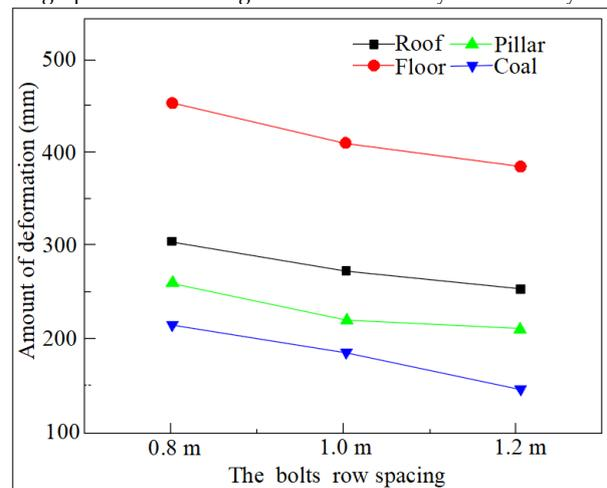
(b) Displacement graph of surrounding rock in the roadway with an interlayer spacing of 2.5 m
