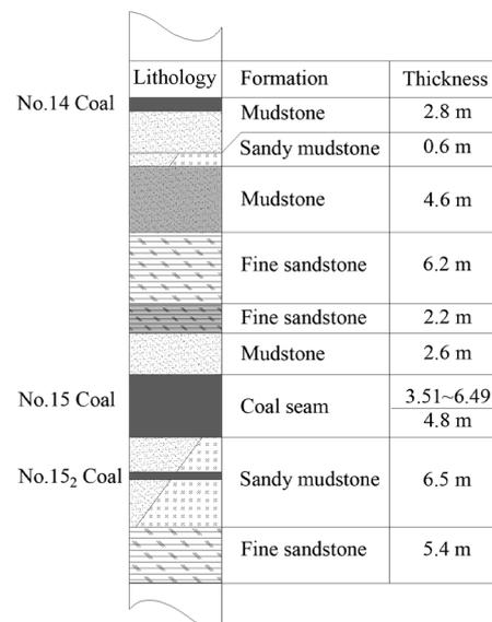
**Figure 5.** Lithological column of the Ping'an Coal Mine.
