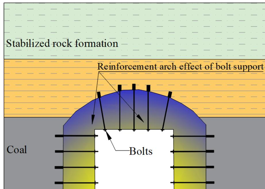
**Figure 3.** Reinforcement arch effect of bolt support.
