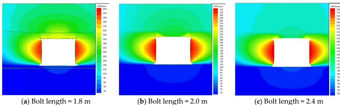
**Figure 11.** Distribution characteristics of the surrounding rock displacement at different bolt lengths.
