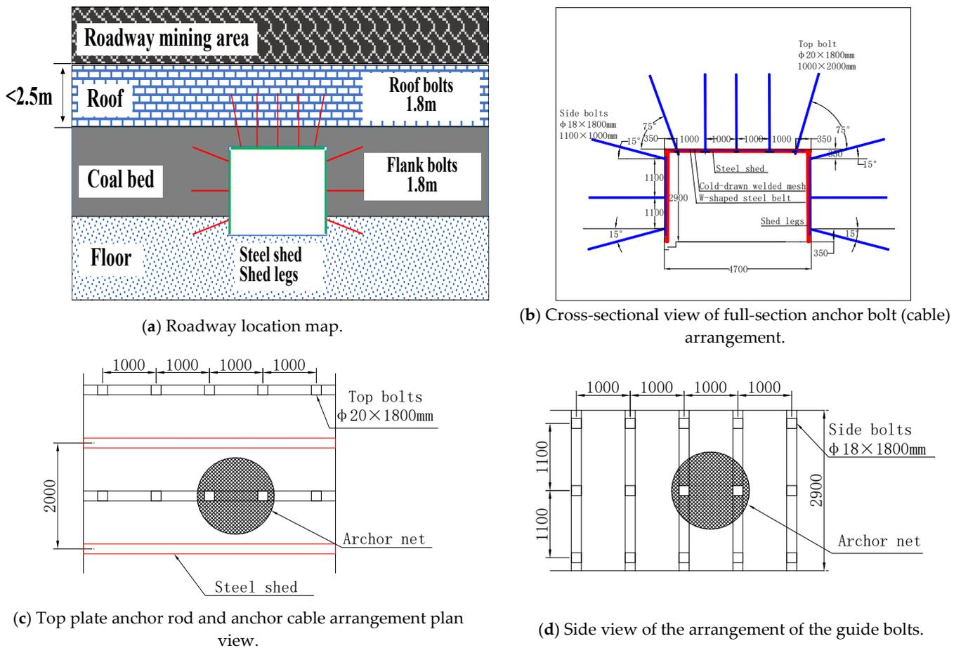
**Figure 20.** Support form for layer spacing less than 2.5 m: (a–d).
