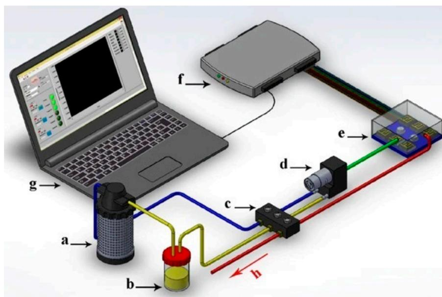
**Figure 2.** Schematic of E-nose used. The components of this system consist of the following parts: (a) Air filter (activated charcoal to remove ambient-air VOC hydrocarbons); (b) Sample headspace chamber; (c) Solenoid air valves; (d) Diaphragm pump; (e) E-nose sensor array chamber; (f) Data acquisition recorder; (g) Personal computer (PC); (h) Air outlet line from sensor array chamber (for exhaust gases) [37].
