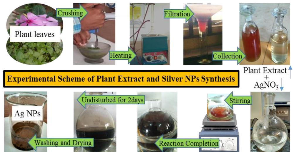
**Figure 1.** Experimental design for synthesis of Ag NPs using *O. tenuiflorum* and *C. roseus*.
