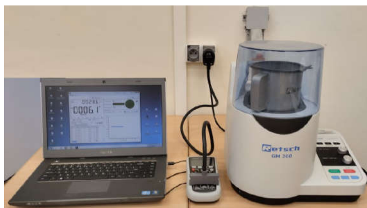
Figure 1. Measuring stand for the recording of grinding energy of triticale grain.
