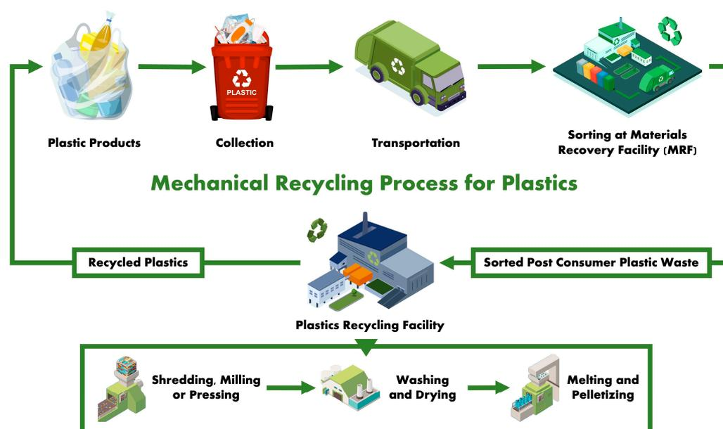
**Figure 3.** Modern mechanical recycling process for plastic waste.
