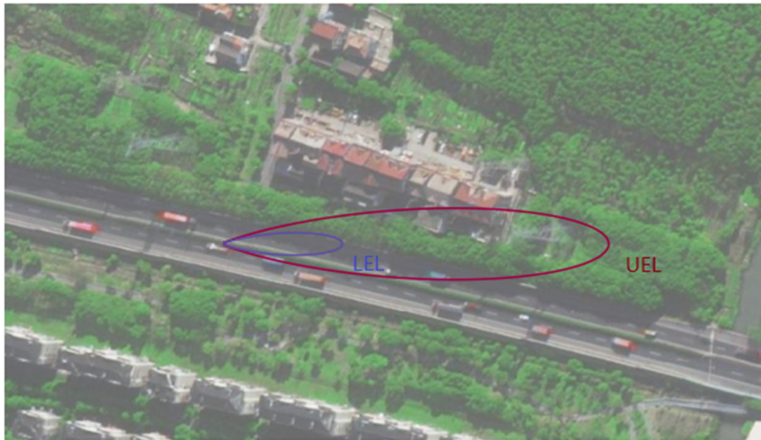
Figure 12. The concentration distribution of gas diffusion (3 min, d = 0.0508 m).
