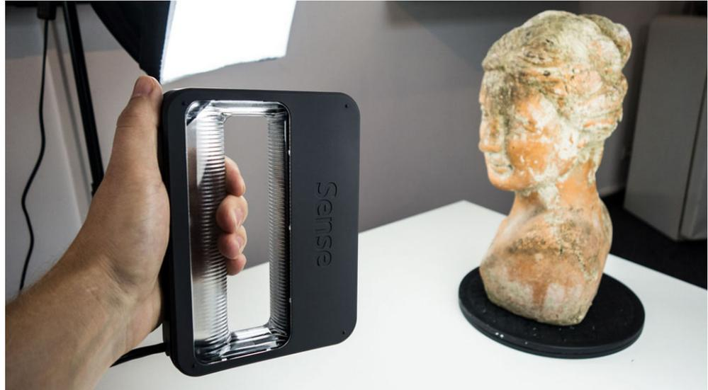
**Figure 2.** Handheld 3D scanner apparatus.
