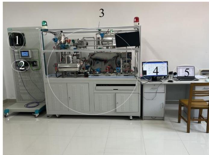
**Figure 17.** Experimental equipment and devices: 1. SIMATIC S7-400 PLC; 2. ET200M; 3. SMPT-1000 experiment platform; 4. Industrial control machine monitor; 5. Upper computer.
