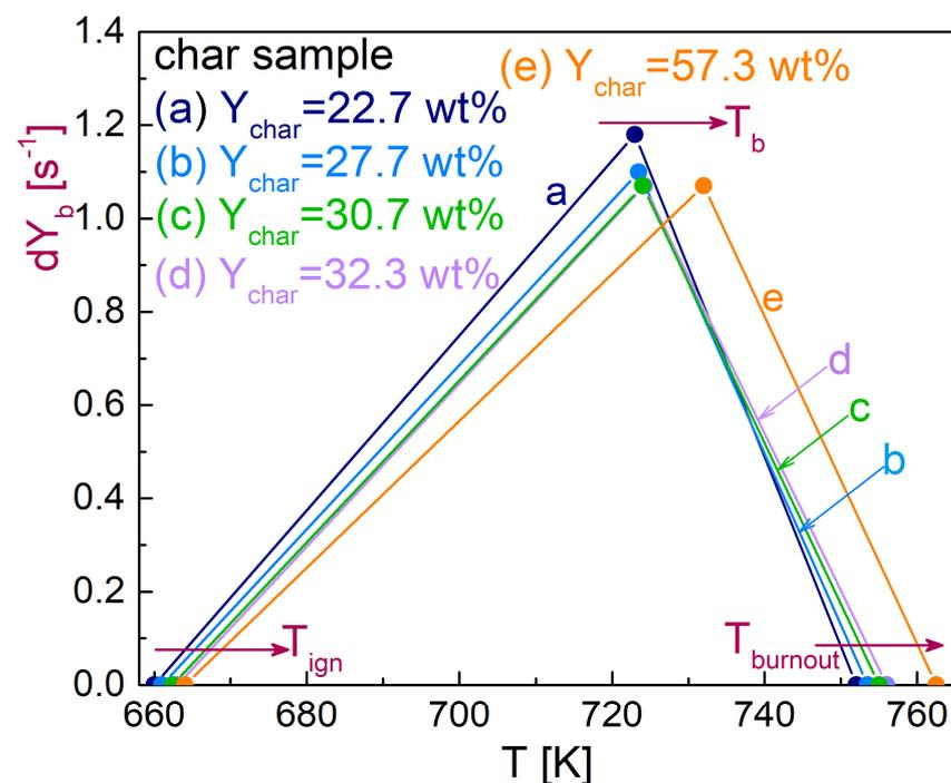
**Figure 4.** Peak rate versus temperature, using the three characteristic values,  $T_{\text{ign}}$ ,  $T_b$  and  $T_{\text{burnout}}$ , for the various char samples (torrefaction conditions as shown in Table 1).
