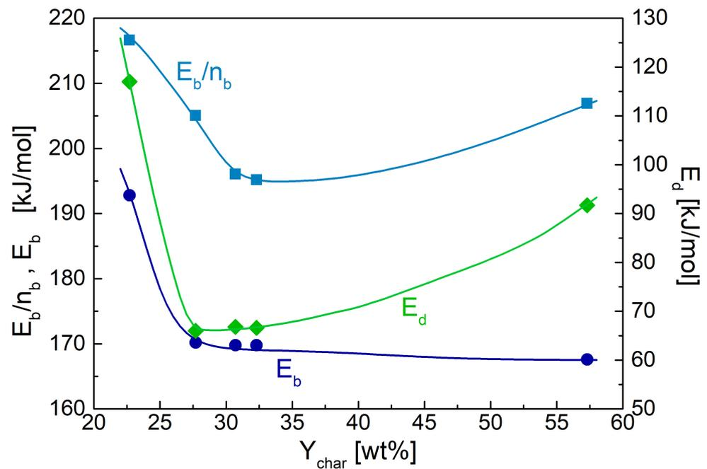
**Figure 5.** Activation energies of the devolatilization reaction,  $E_d$ , and the oxidation reaction,  $E_b$ , and ratio  $E_b/n_b$  ( $n_b$  reaction order) versus the torrefaction degree expressed in terms of pyrolysis char yield,  $Y_{char}$ .
