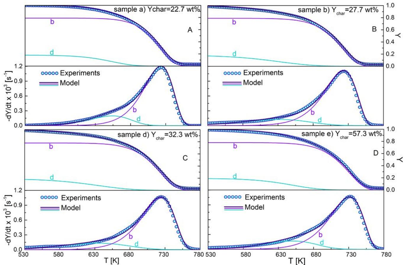
**Figure 6.** Weight loss curves ( $Y$ ) and devolatilization rate curves ( $-dY/dt$ ) for the pyrolysis chars samples a (A), b (B), d (C) and e (D) (torrefaction conditions in Table 1) versus temperature, as measured (symbols) and predicted (solid lines) (including the prediction for the devolatilization (d) and oxidation (b) reactions).
