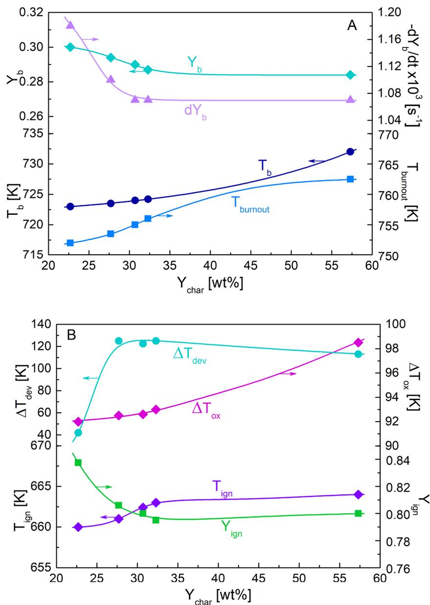
**Figure 3.** Thermogravimetric parameters  $dY_b$ ,  $T_b$ ,  $Y_b$ ,  $T_{burnout}$  (A), and  $T_{ign}$ ,  $Y_{ign}$ ,  $\Delta T_{ox}$  and  $\Delta T_{dev}$  (B), versus the torrefaction degree expressed in terms of pyrolysis char yield,  $Y_{char}$ .
