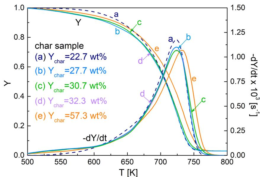
**Figure 1.** Weight loss curves (Y) and devolatilization rate curves ( $-dY/dt$ ) as functions of temperature for the oxidation of fixed-bed chars produced at 800 K, from untreated and torrefied spruce wood (torrefaction conditions in Table 1) measured for a heating rate of 5 K/min.
