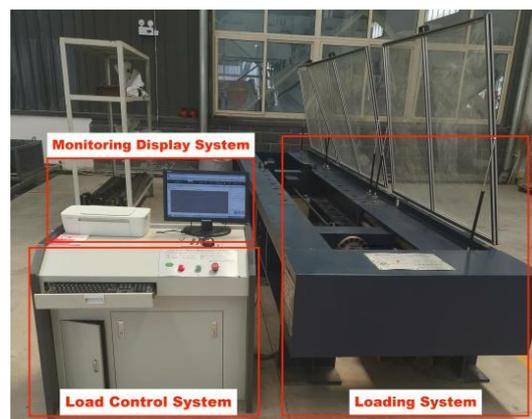
**Figure 4.** 600 KN anchor static load test system.
