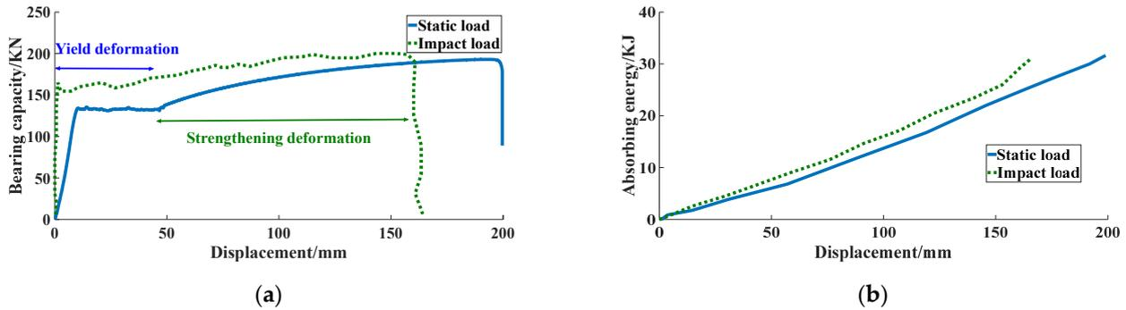
Figure 10. Mechanical property curves of conventional anchor rods (a) bearing capacity-displacement curve; (b) energy absorption characteristic curve.
