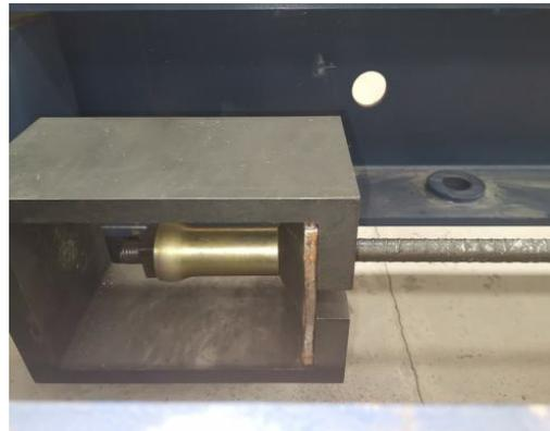
**Figure 6.** The energy absorbing anchor static load tensile test.
