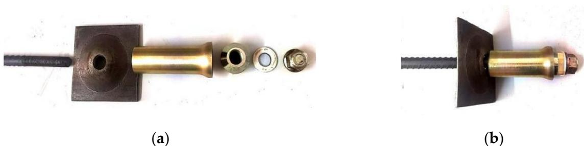
**Figure 2.** The actual structure of energy absorbing anchor (a) before assembly; (b) after assembly.
