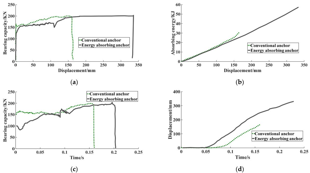
**Figure 12.** The comparison of the mechanical property curves of conventional anchor and energy absorbing anchor: (a) bearing capacity–displacement curve; (b) energy absorption characteristic curve; (c) bearing capacity–time curve; (d) displacement–time curve.
