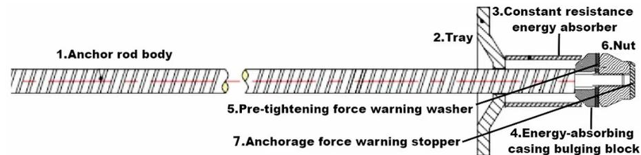
**Figure 1.** Energy absorbing anchor structure diagram.
