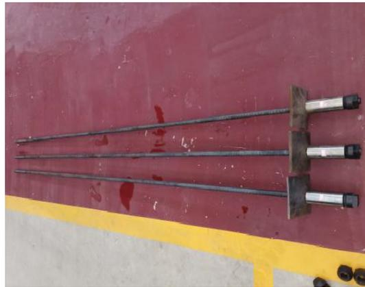
**Figure 3.** Energy absorbing anchor.
