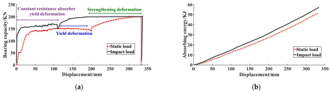
Figure 11. Mechanical property curves of energy absorbing anchor rods (a) Bearing capacity-displacement curve; (b) Energy absorption characteristic curve.
