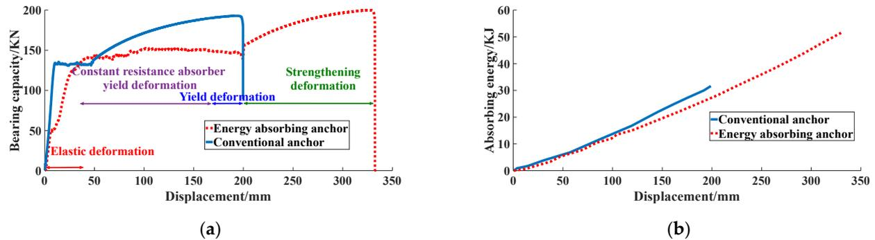
**Figure 8.** The comparison of the mechanical property curves (a) bearing capacity-displacement curve; (b) energy absorption characteristic curve.
