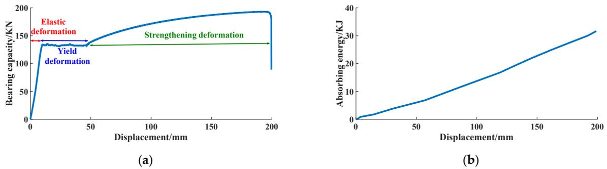
**Figure 5.** Mechanical property curves of conventional anchor rods (a) Bearing capacity-displacement curve; (b) Energy absorption characteristic curve.
