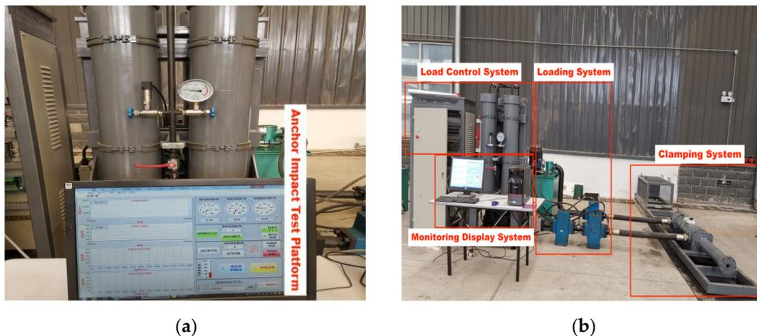
**Figure 9.** 300 kN anchor impact test system (a) Anchor impact test platform; (b) Anchor impact test bench.
