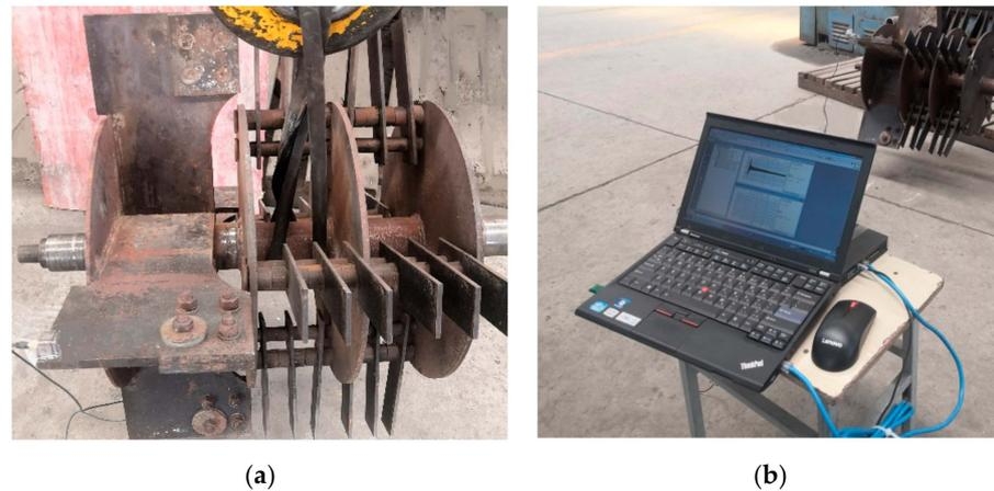
**Figure 12.** Site of the steel ball impact vibration test. (a) Sensor placement; (b) steel ball impact vibration test system.
