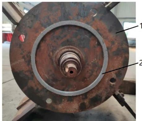
**Figure 11.** Installation position of the support plate damping ring. (1) Support plate; (2) damping ring.
