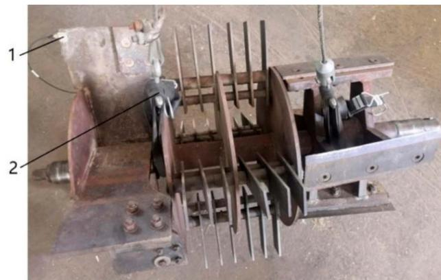
**Figure 2.** Modal test layout. (1) Suspension point; (2) sensor placement point.
