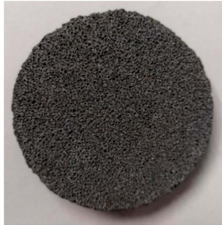
**Figure 8.** Microcellular foam aluminium material.
