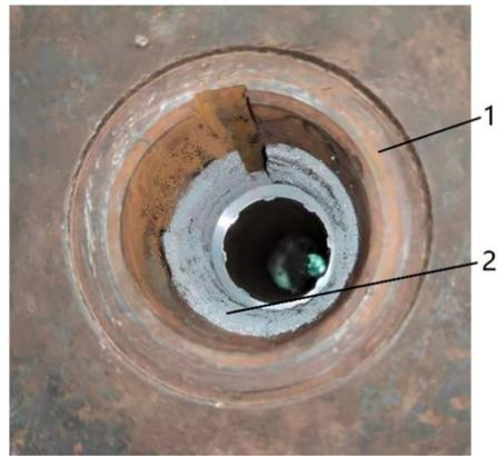
**Figure 10.** Mounting position of the damping ring of the hob shaft sleeve. (1) Hob shaft sleeve; (2) damping ring.
