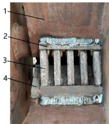
**Figure 9.** The installation position of the foamed aluminium material of the throwing blade. (1) Throwing blade; (2) steel plate; (3) triangular aluminium foam; (4) square aluminium foam.
